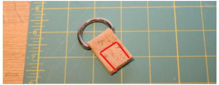
118. Slip your strap through the D-ring, fold your strap in half with raw edges together. Sew the ends together as shown with red lines above.
