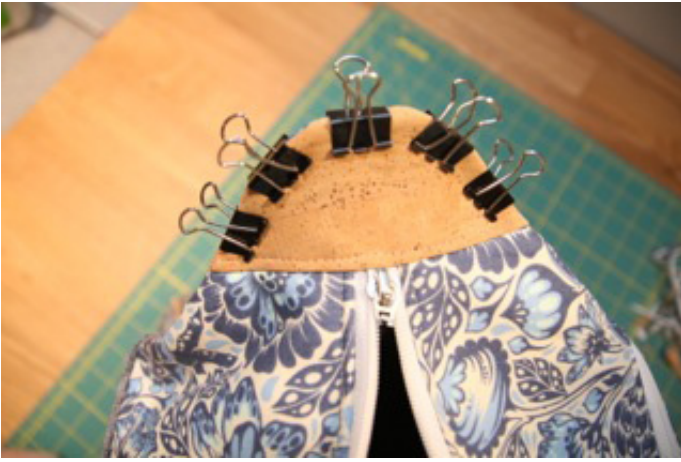
109. Smooth and flatten your rounded connector seam and clip in place with the peltex piece sandwiched inside.
