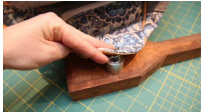
113. Flip your bag so you have the WS of your connector facing up. Place the post half of your grommet through the hole and all the layers from the RS. Place that half of your grommet on your anvil. Place the grommet's washer over the post.
