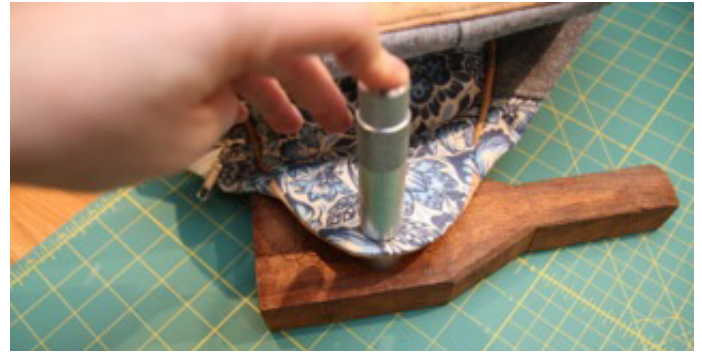
114. Gently hammer your setter to set your grommet. Repeat steps 111-114 for second connector.
