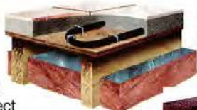
Thin Slab Over Frame Floor Heating
