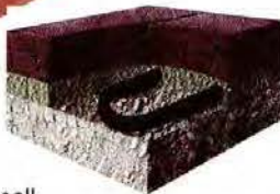
Brick Paver Snowmelting
