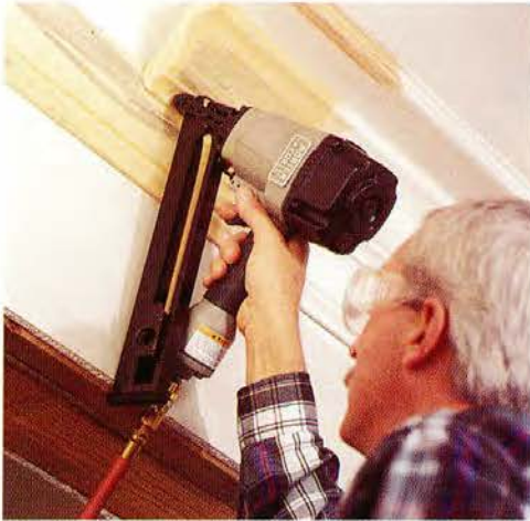
DA250A Angle Nailer - Ideal for crown molding, shoe molding and upholstery trim boards in furniture.
