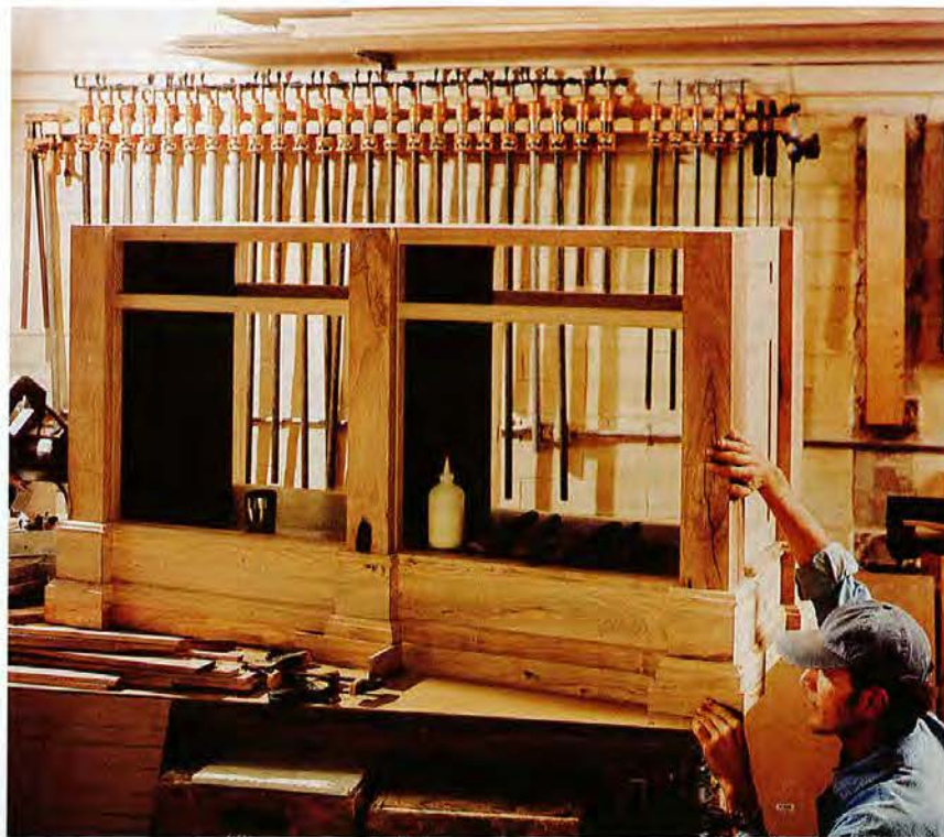
Cabinetmaker James Vosnos assembles the frame of the Meigses’ kitchen island, which has an epoxy-filled knothole prominently displayed in the center pilaster. “That’s why people like mesquite,” Vosnos says. “It tells a story.”
