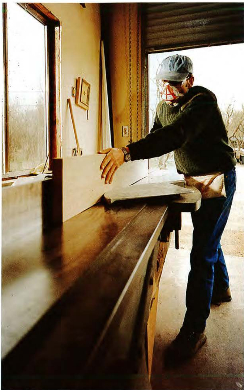
Mesquite is a tough, ornery wood to work with, so Vosnos is always ready for trouble as he pushes a plank across his jointer. Mesquite is so hard it dulls the jointer blade twice as fast as any other wood.
