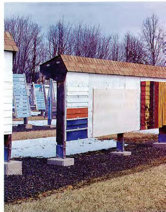
At the Paint Quality Institute near Philadelphia, odd-looking fences test how paint performs on wood, aluminum and even faded vinyl siding.
