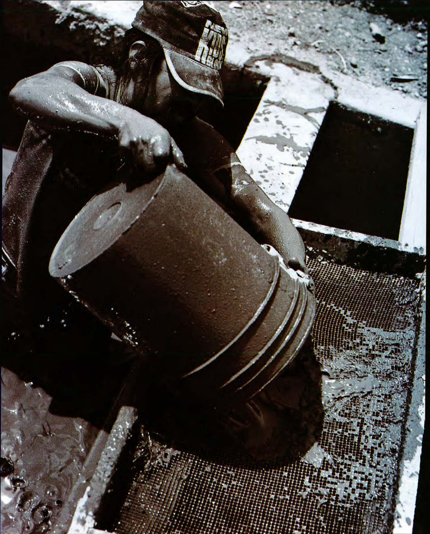
Fortino Ramirez filters mud that workers will knead with their bare feet and turn into malleable clay.
