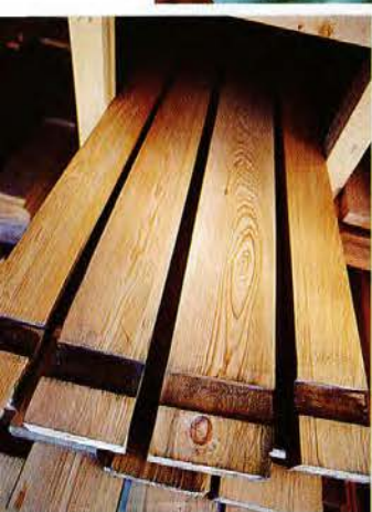
ABOVE: In Killen's Death & Resurrection millwork shop, Gerald Lendway builds an exterior door out of cypress, the wood of choice to withstand Nantucket's blowing rains. LEFT: Killen's precious stockpile of cypress staves salvaged from a brewery's vats.
