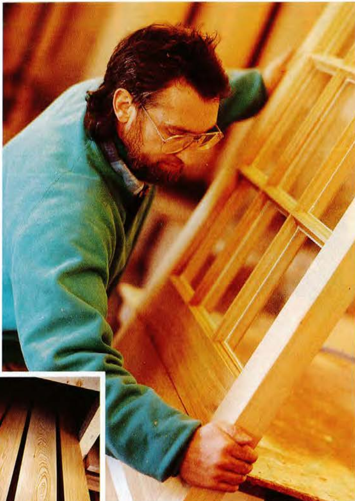
ABOVE: In Killen's Death & Resurrection millwork shop, Gerald Lendway builds an exterior door out of cypress, the wood of choice to withstand Nantucket's blowing rains. LEFT: Killen's precious stockpile of cypress staves salvaged from a brewery's vats.
