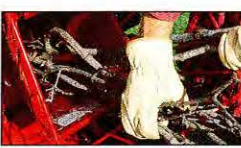
Chipping Chute feeds branches into blade spinning at 3,600 rpm.
