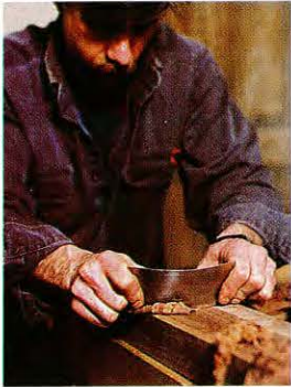
Denis Semprebou demonstrates. Scrapers are a favored tool at the Boston-based school, where Semprebou teaches preservation carpentry. His students learn to repair this country's oldest buildings.
