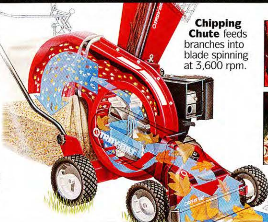
Auto-fill Bag neatly contains the pulverized leaves; holds 3 1/2 bushels.
