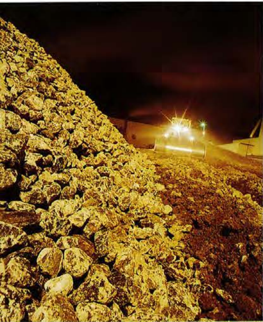
Raw gypsum rock fresh from a Nova Scotia quarry awaits the crusher, the next step on its way to becoming drywall.
