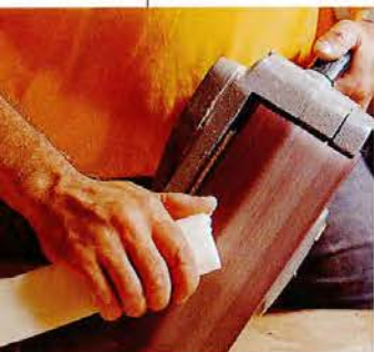
When grit clogs, Tom Silva erases the residue with a rubber cleaner held against the belt. He makes sure to keep his fingers clear.
