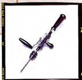
Hand drill: The egg-beater design works with small-diameter bits. For larger holes, use a brace.
