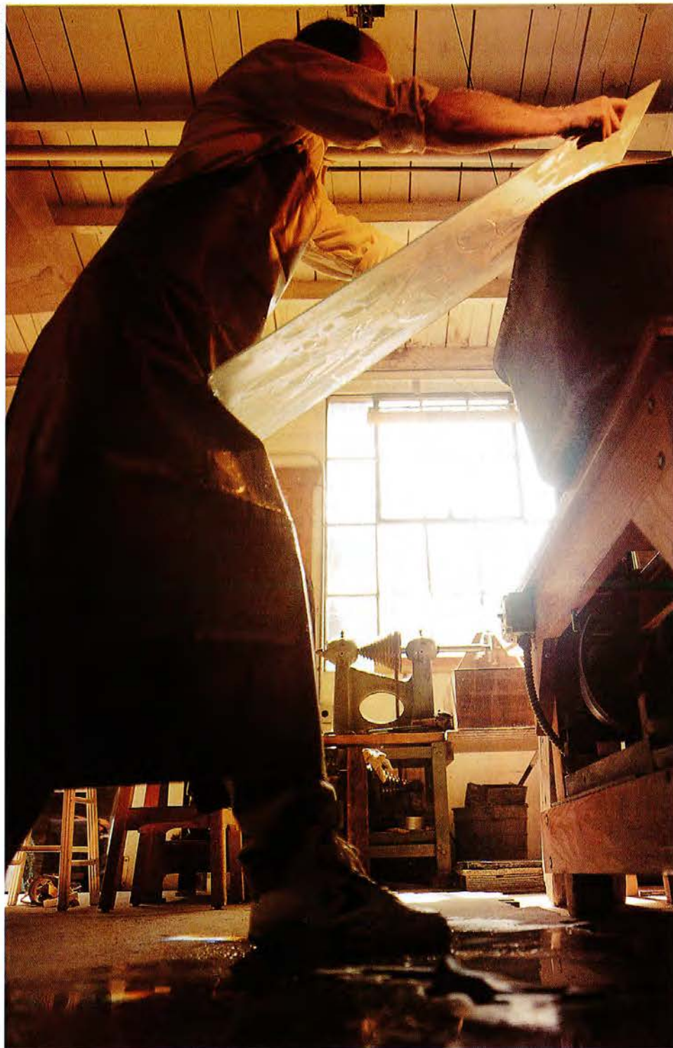
Using his body as a brace, Lehmann pushes the glass against a whirling abrasive wheel.
