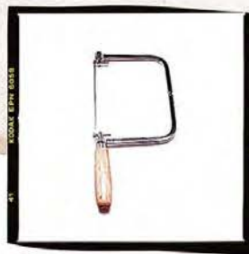
Coping saw: Good for curves. For cutouts, remove the blade, thread it through a hole in the wood, then reattach blade to handle.
