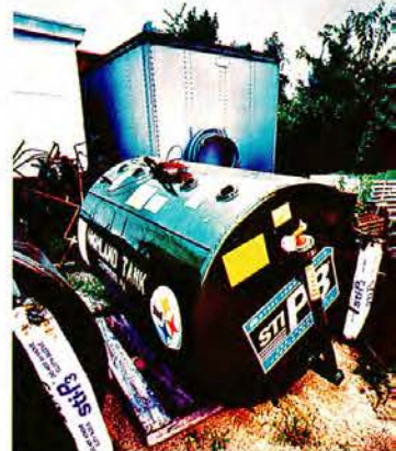
The STIP3 tank has a sacrificial zinc anode hanging from it like a white buoy.
