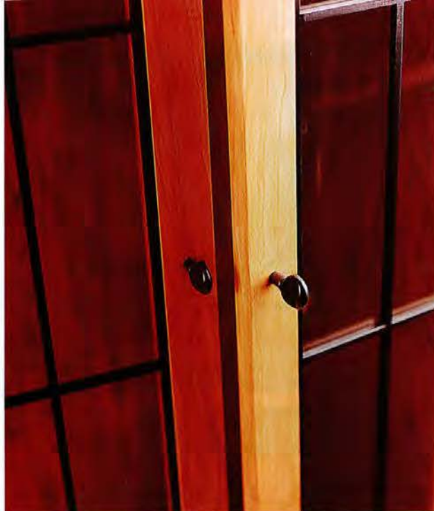
Seward can spend hours deciding how the grain should run throughout a piece. Here, the inside stiles of a cherry library cabinet door are book-matched and accented with black viola tuning pegs and mullions dyed black for a richer color.
