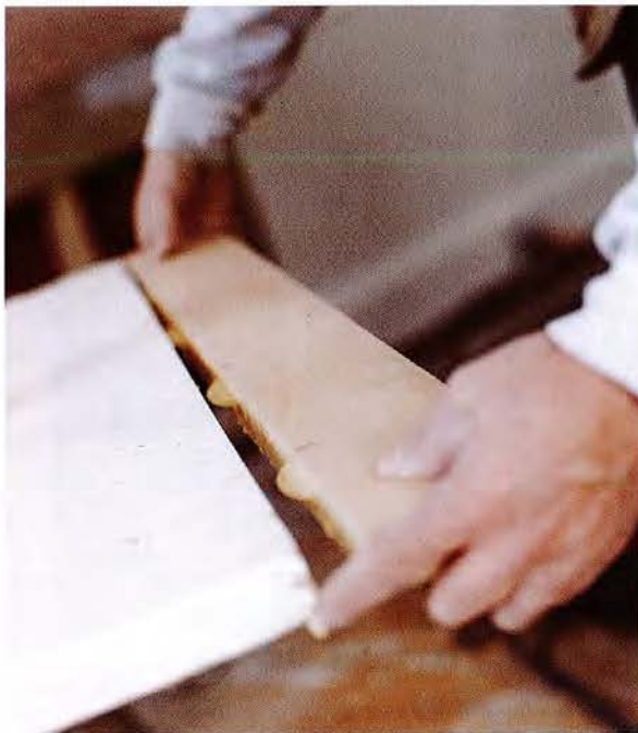
Biscuit joints guarantee a strong bond and create a good alignment for the filler piece Silva edge-glues to the door's bottom.
