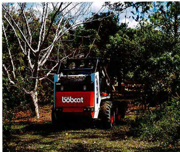
Hydraulic drives on each side allow these earth-movers to thread nimbly among obstacles that might stymie bigger machines.
