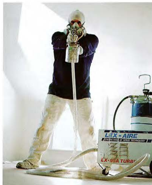
Dee's deluxe HVLP system features a 2.5-gallon pressure pot (atop the turbine), big enough to hold an open can of paint. This option increases capacity, reduces cleanup and refill time and lightens the spray gun—an important consideration when spraying overhead.
