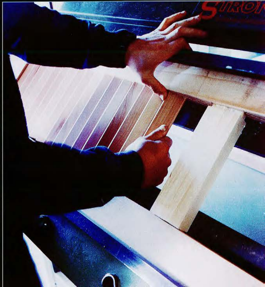
than 72 inches long or 18 inches wide, they're assembled with dowels like these, two at each joint. Larger shutters are made with stronger mortise-and-tenon joinery. BELOW RIGHT: Assembler Mike Cresswell inserts louvers with a practiced snap. When all are in place, he'll squeeze the shutter together in a pneumatic press that develops 120 pounds per square inch of pressure.
