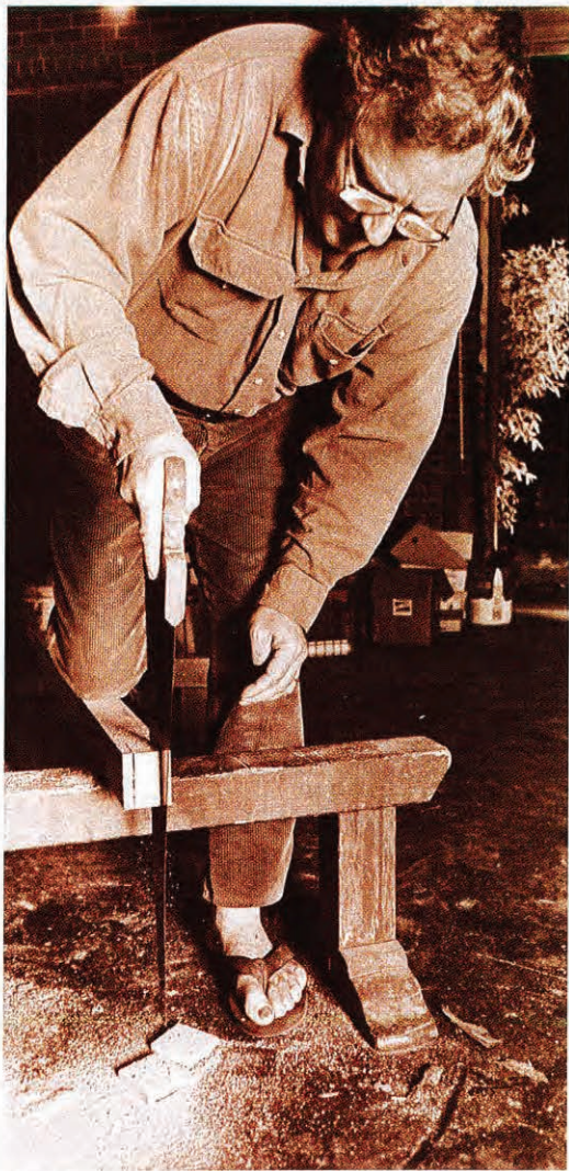
The push stroke of the Western ripsaw requires strength and control in one arm—and puts a lot of strain on it. Here, Discoe's body weight is to the left of the line of cut.
