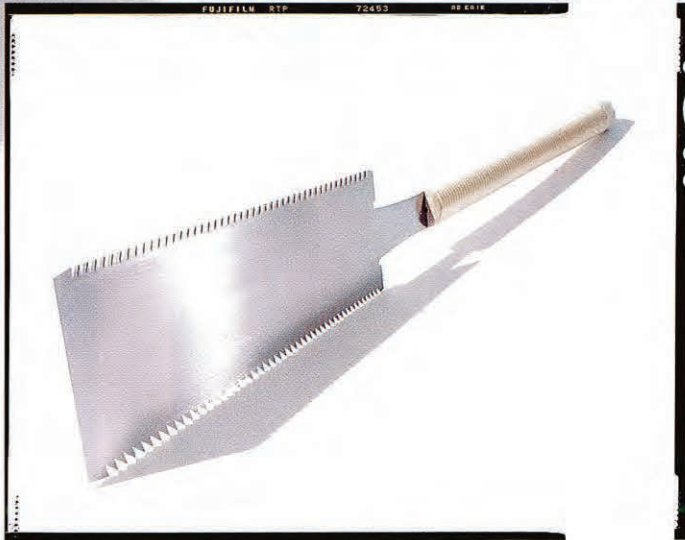
BELOW: This ryoba noko giri has 10 crosscut teeth per inch on one edge, 5 rip teeth per inch on the other. Rip teeth increase in size from the heel (near the handle) to the toe of the blade, while all crosscut teeth are identical.
