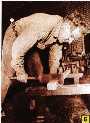
He finishes with the saw level, then flips the piece over for the final cut. He stays just outside of the line so the tenon is a bit larger than it needs to be. Typically, these rough cuts are finished with a Japanese chisel for a tight fit of mortise and tenon.
