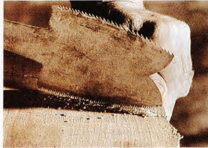
LEFT: The azebiki noko giri is designed for cutting mortises, grooves in midpanel and sliding dovetails, like the one pictured above. It is especially useful when the craftsman must maneuver in a tight area without damaging adjacent work.
