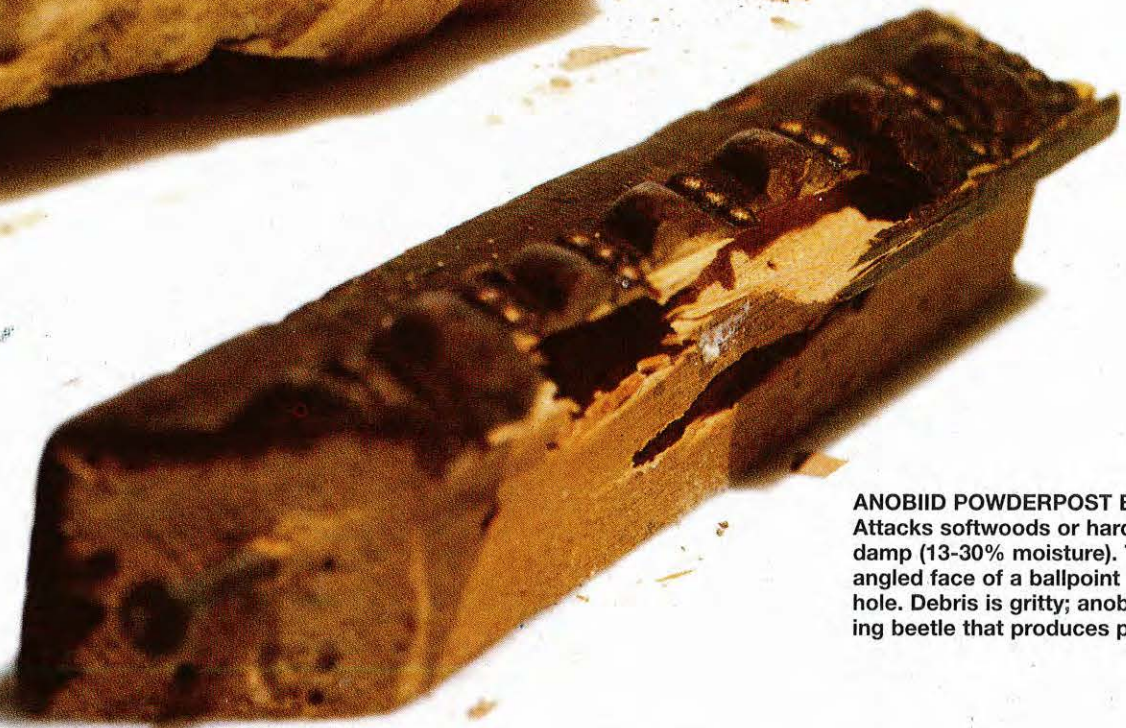
OLD HOUSE BORER Round-headed larvae leave rippled gallery walls. Old house borer eats only sapwood of softwoods, primarily pine. Debris is tightly packed.
