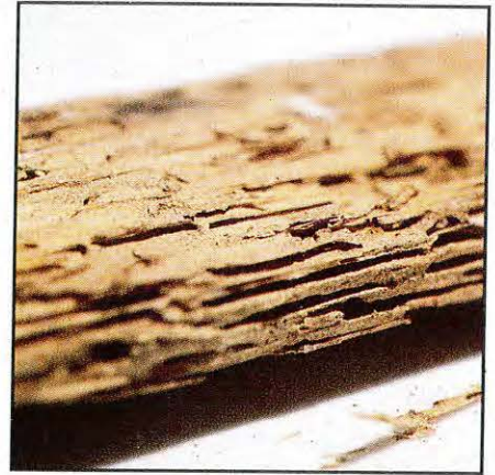
SUBTERRANEAN TERMITE Eats only soft spring growth, so wood has layered appearance. Gritty mixture of mud, saliva and fecal matter is common inside galleries. No pellets.
