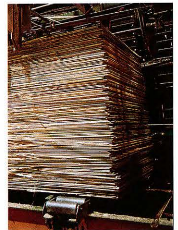
Stacks of raw plywood emerge from the press, ready for trimming. The heated press sets the glue in minutes, welding the veneers together.
