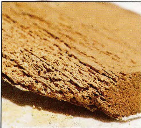
LYCTID POWDERPOST BEETLE Eats hardwoods only. Wood can be dry to moist (8-32% moisture). Only tip of ballpoint pen fits in exit hole. Debris feels like talc, is loosely packed and contains no pellets.
