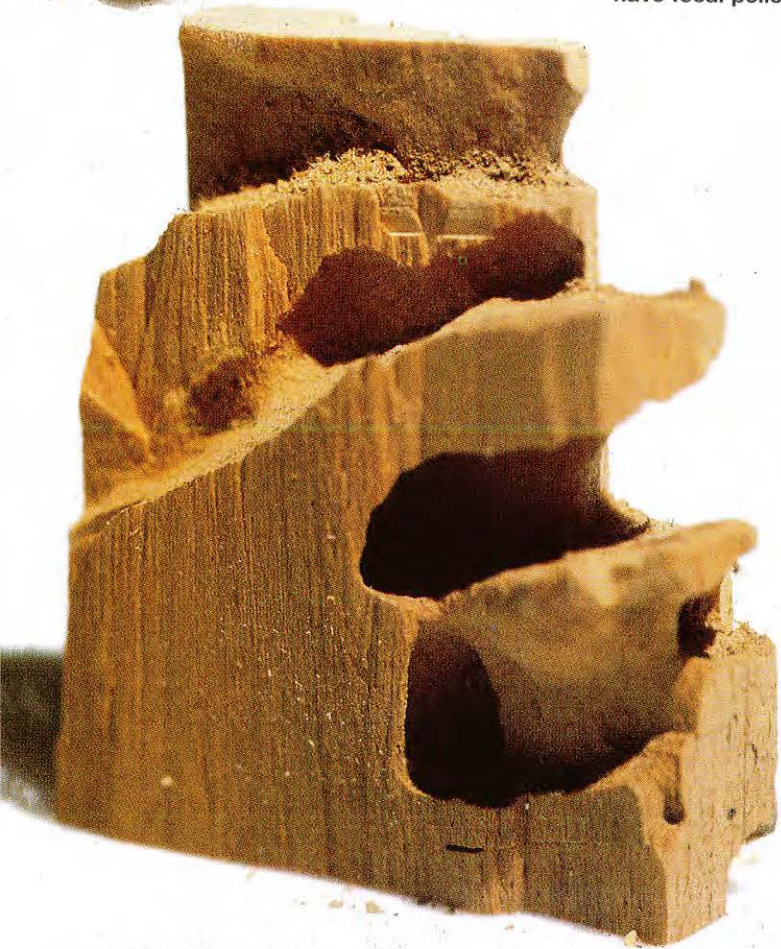
CARPENTER ANT Galleries follow soft spring growth, with numerous connections through the harder, darker summer wood. Galleries are free of debris. Surface often contains holes through which the ants push out wood shavings and uneaten parts of insects.
