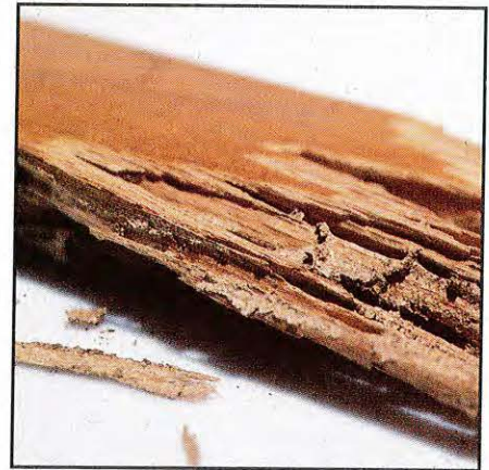
FORMOSAN TERMITE Damage is similar to that of other subterraneans, but galleries also contain carton, a nesting material that looks like sponge but is hard.
