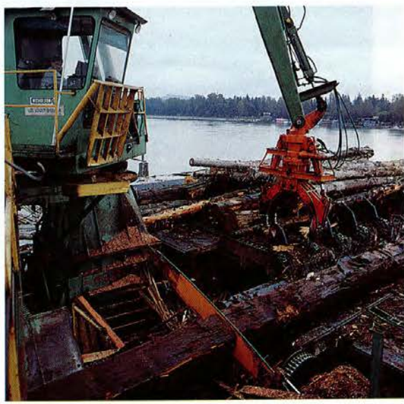
An 8-foot automated chain saw "bucks" each log down to millable 20-foot lengths.
