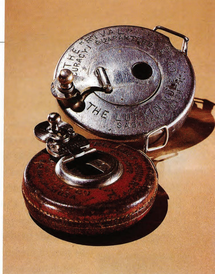
Before self-retracting steel tapes, hand-cranked models measured long distances. "Reliable Junior" of 1893 has a leather case and pop-out winding handle. "The Rival" is newer. Both measure 25 feet.
