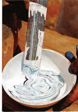
A bit of blue in a bowl of white titanium dioxide paint.
