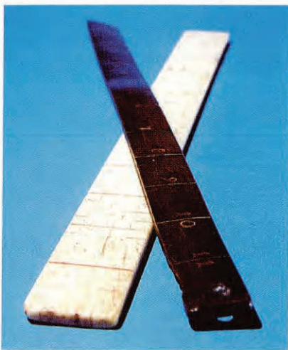
Rules continued to be handmade even after factories opened. Nineteenth-century whalers carved these, in bone and black baleen.
