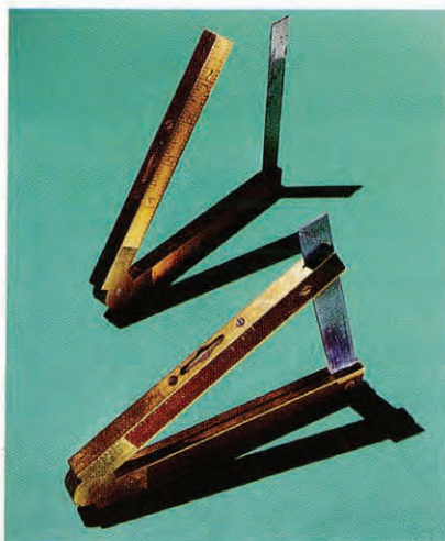
Made of ebony and boxwood with brass, these 12-inch, two-fold rules also are equipped to be levels, inclinometers, squares and bevels.
