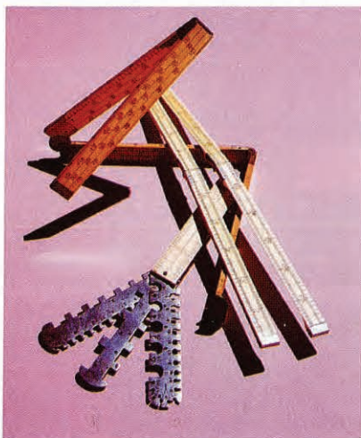
Rules with math aids, from top: built-in board-measure table, architect's scales, wire and iron gauges.
