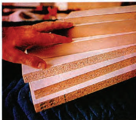
Compare 1-inch-thick MDF (top three boards) with 3/4-inch particleboard (lower three).
