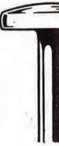
Pan Wide head allows for increasing strength. Not so usually used where
