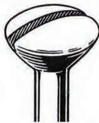
Slotted Useful now mostly on antiques, where other options would look out of place.
