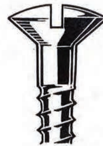
Oval Used where appearance counts. Back bevel allows most of head to be countersunk.
