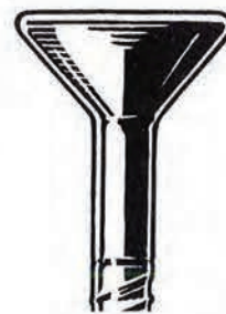
Flat Designed to be countersunk so top sits flush. For neat job, countersink must be predrilled.
