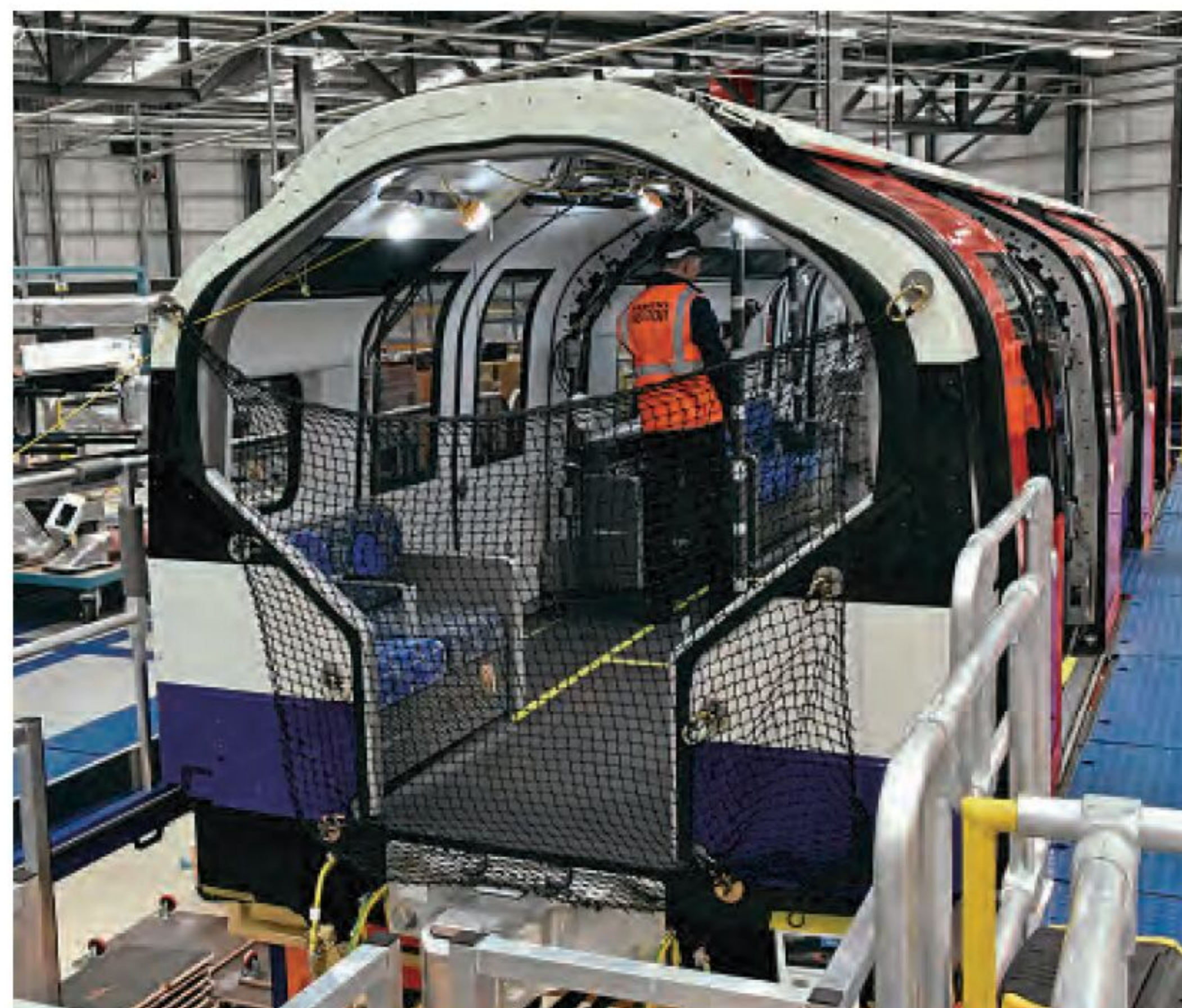
Fitted-out car body No. 94, part of the Piccadilly line order, is seen at Siemens Goole Rail Village on the eve of its official opening, during an event at which members of the media were invited to look around. Bogies are added later in the assembly process. GRAEME PICKERING
