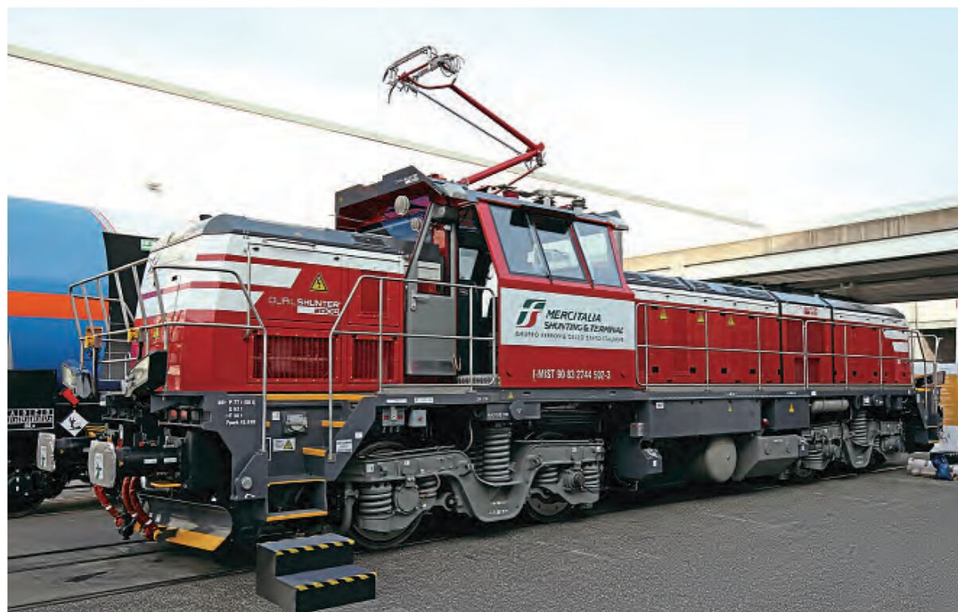
Above: The new 'e6' battery-powered switcher built by Italian manufacturer IPE Railway Vehicles, which uses batteries from Indian firm Medha. KEITH FENDER
