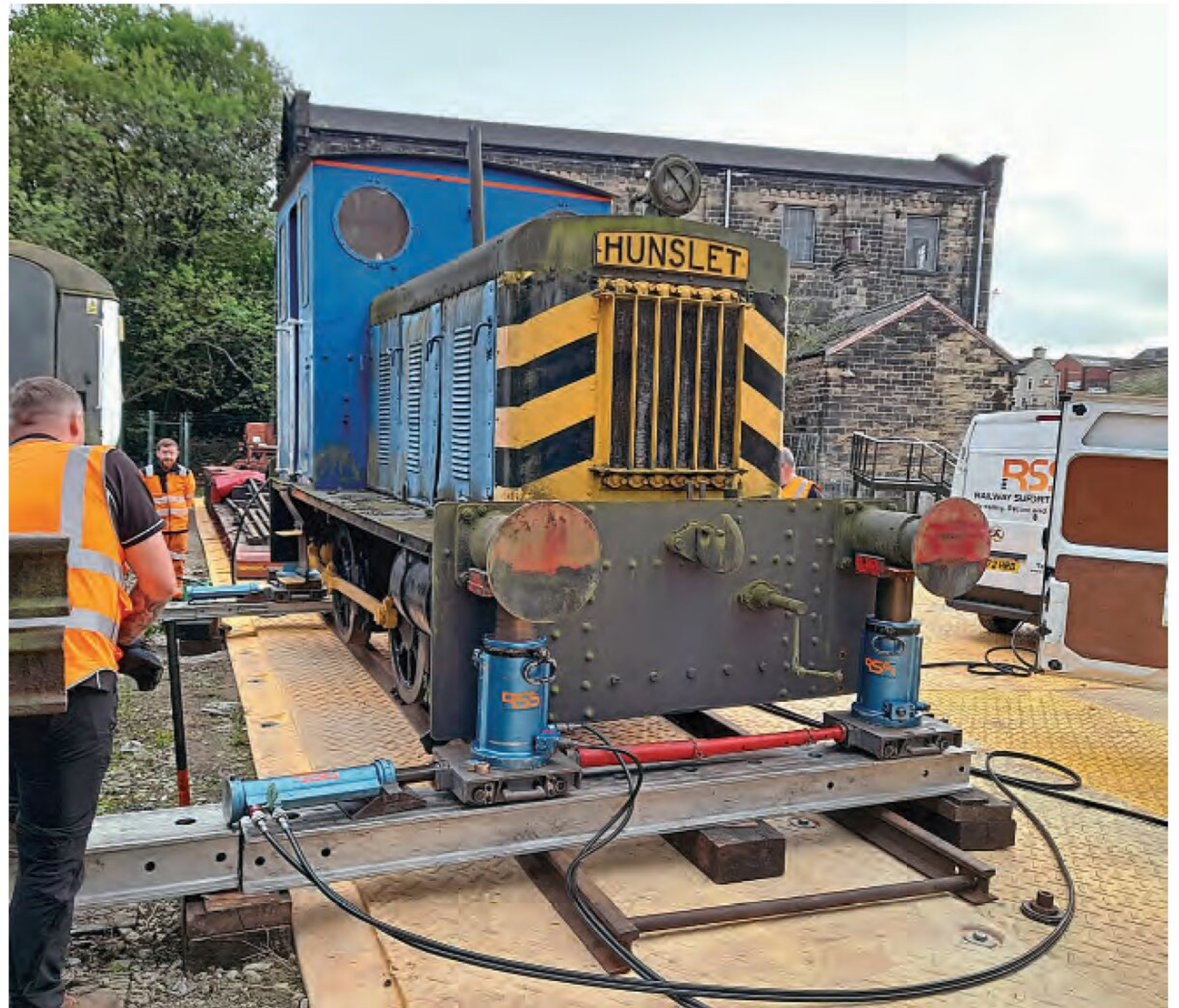
The operation to move Hunslet No. 2641 from the Eureka site in Halifax by jacking it sideways for loading onto a lorry is seen in progress on September 9. It arrived in Preston the following day. STEWART WAUGH
