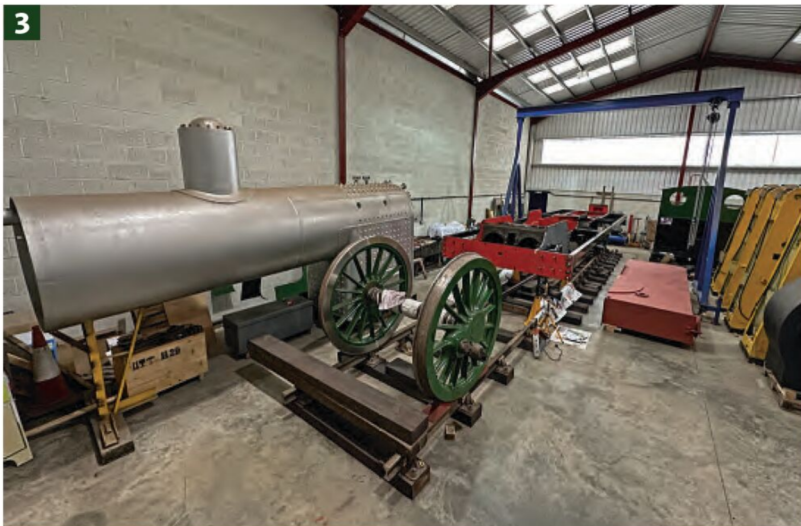
3 The boiler, frames and one set of wheels for new-build 'G5' No. 1759 at the Hackworth Industrial Park in Shildon on September 14.
