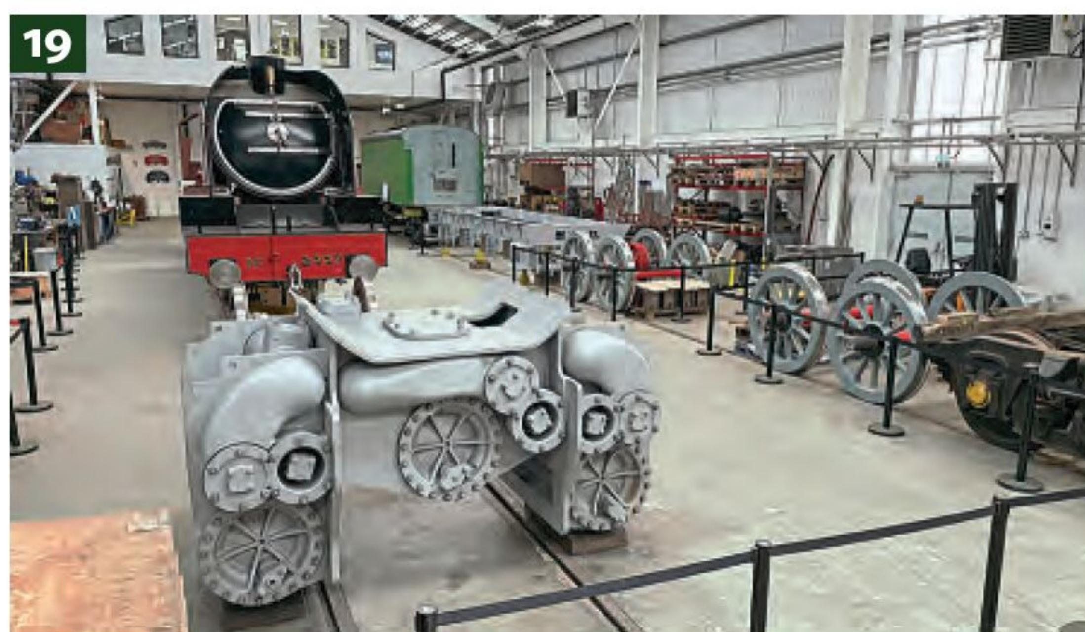
19: A recent view of 'P2' No. 2007 Prince of Wales inside Darlington Locomotive Works. Note the monobloc in front, and the tender frames to the right, which were delivered this summer. A1SLT
