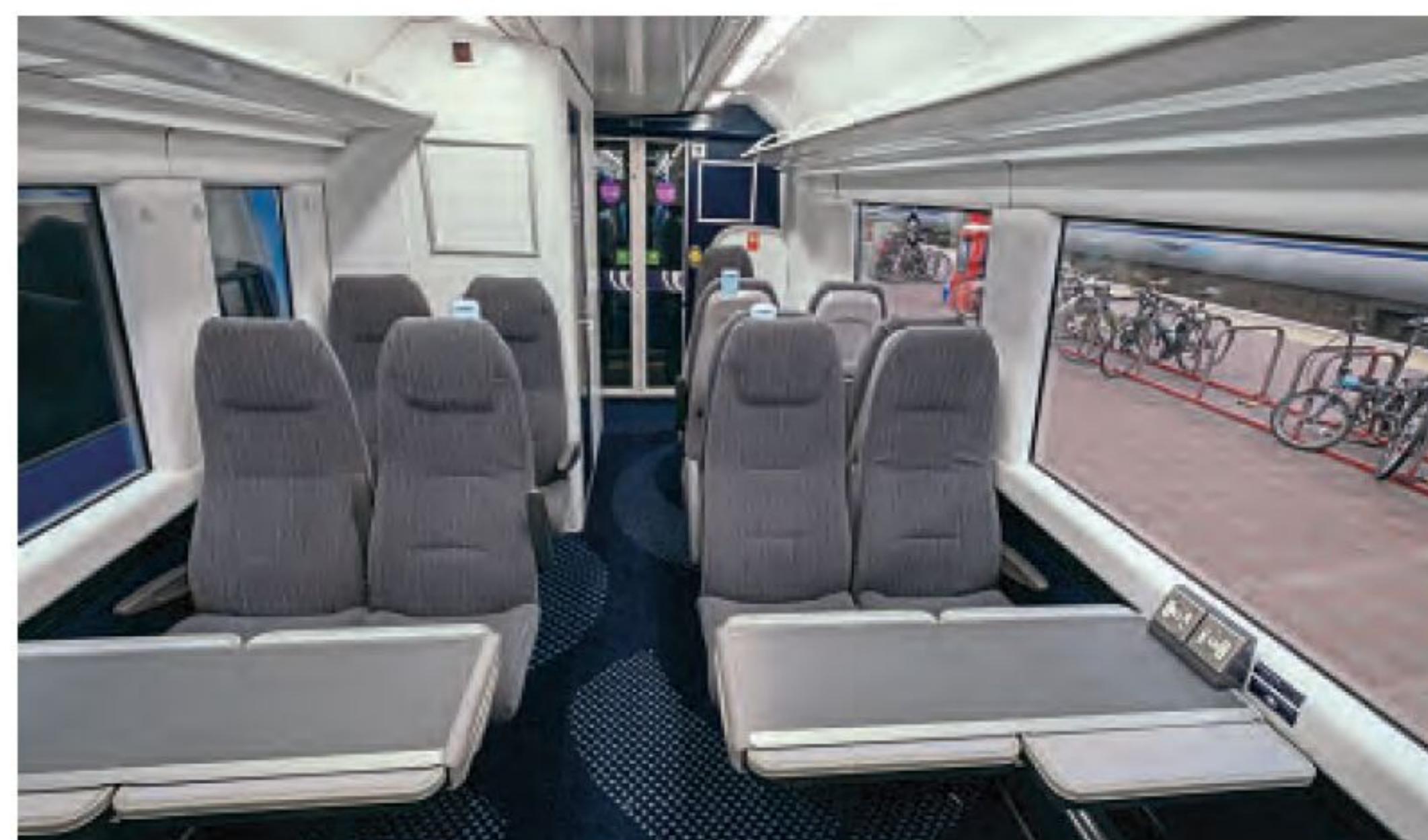
Inside the unit, the refreshed saloon features a grey fleck moquette and new seat cushions. At tables, twin 13-amp sockets with four USB sockets are available, while other seats have a single 13-amp and twin USB. CHRIS MILNER
