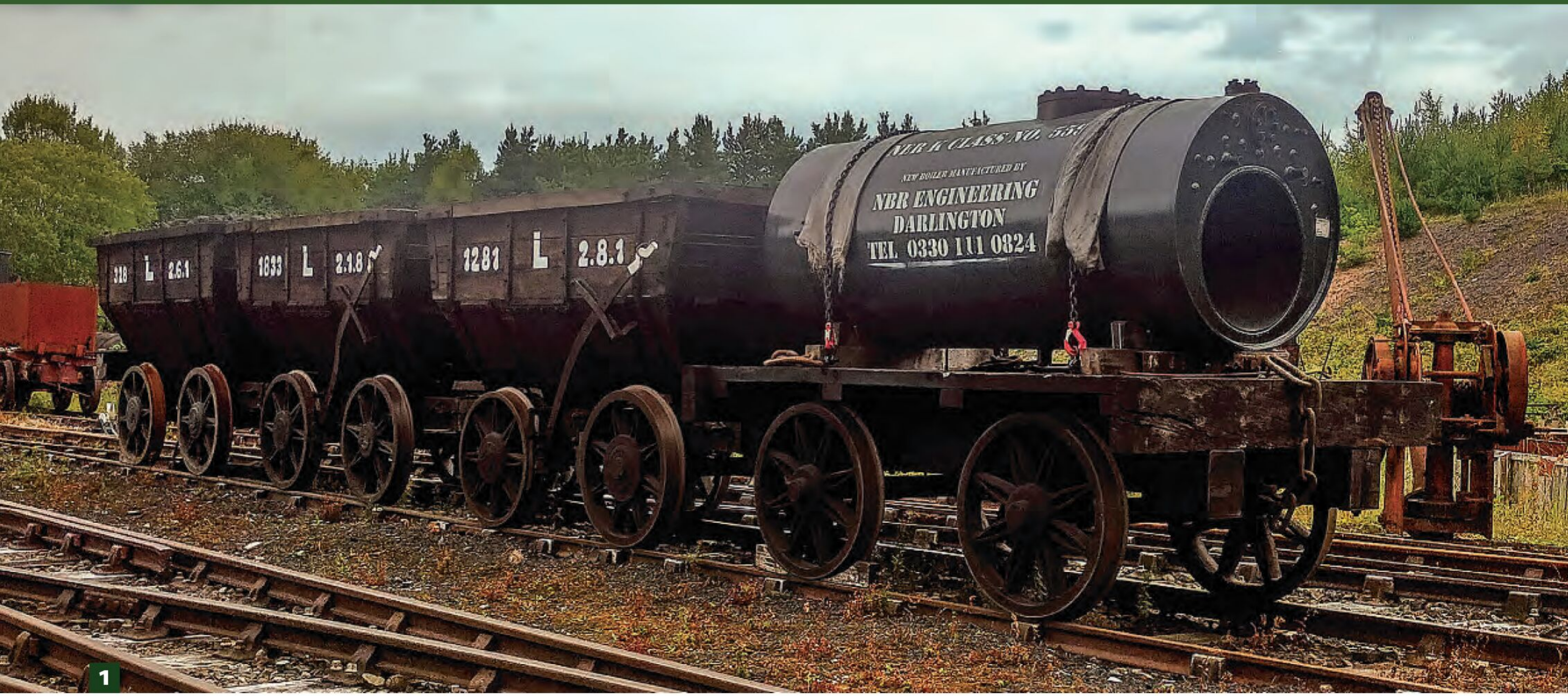
1 Having been completed, tested and painted by North Bay Engineering Services in Darlington, the boiler for new-build NER 'K' 0-4-0T No. 559 arrived at Beamish, The Living Museum of the North, on April 26, 2023. It was then placed onto a flat wagon in the Colliery where it is seen on show on August 19. JAMES GROUNDWATER
