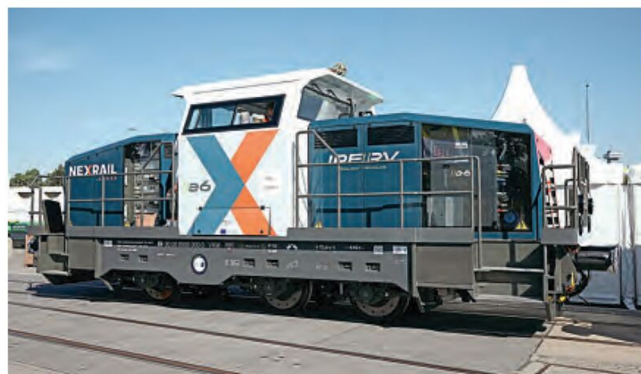
Above: The new 'e6' battery-powered switcher built by Italian manufacturer IPE Railway Vehicles, which uses batteries from Indian firm Medha. KEITH FENDER
