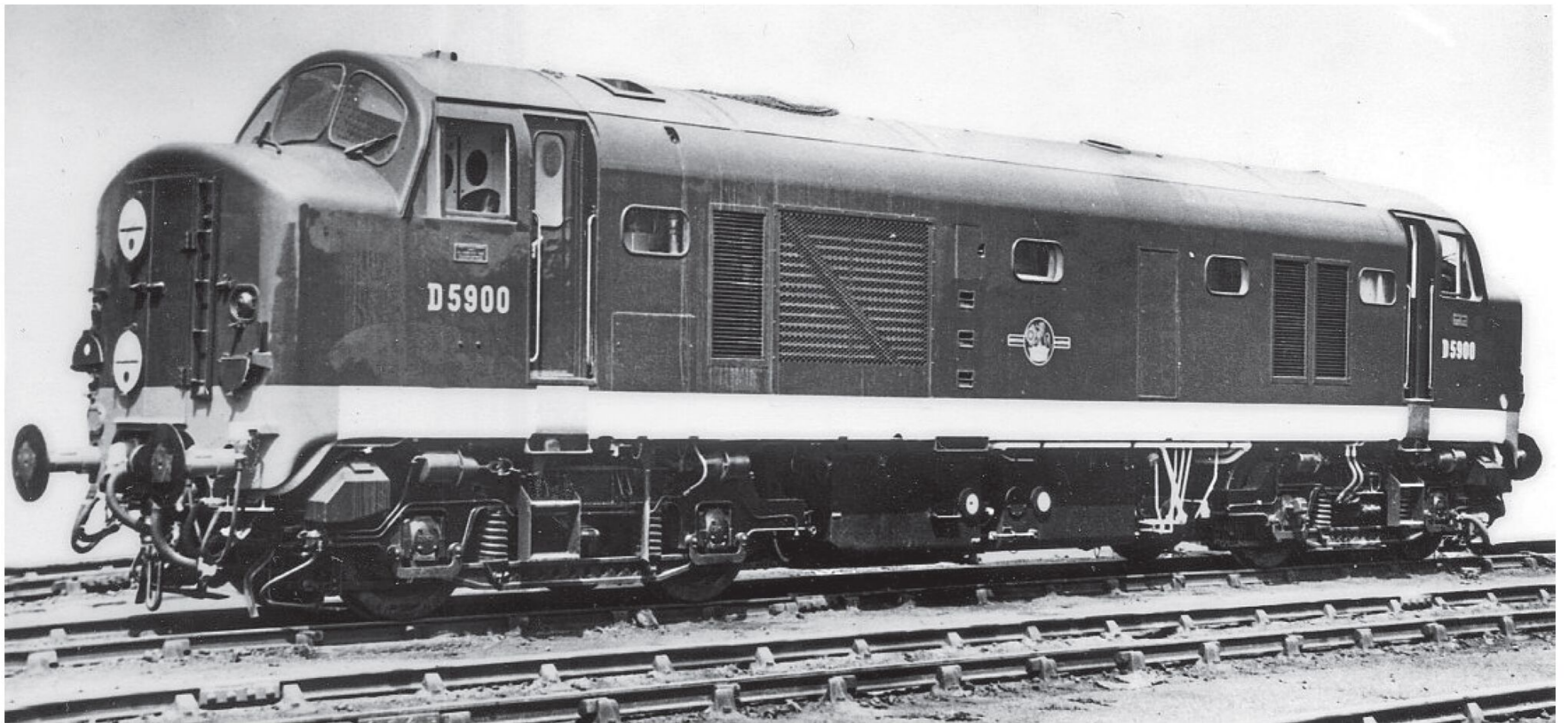
Above: A publicity shot of first-built Class 23 No. D5900 in 1959. They later lost their cab nose gangway and indicator discs in favour of a central headcode box.
