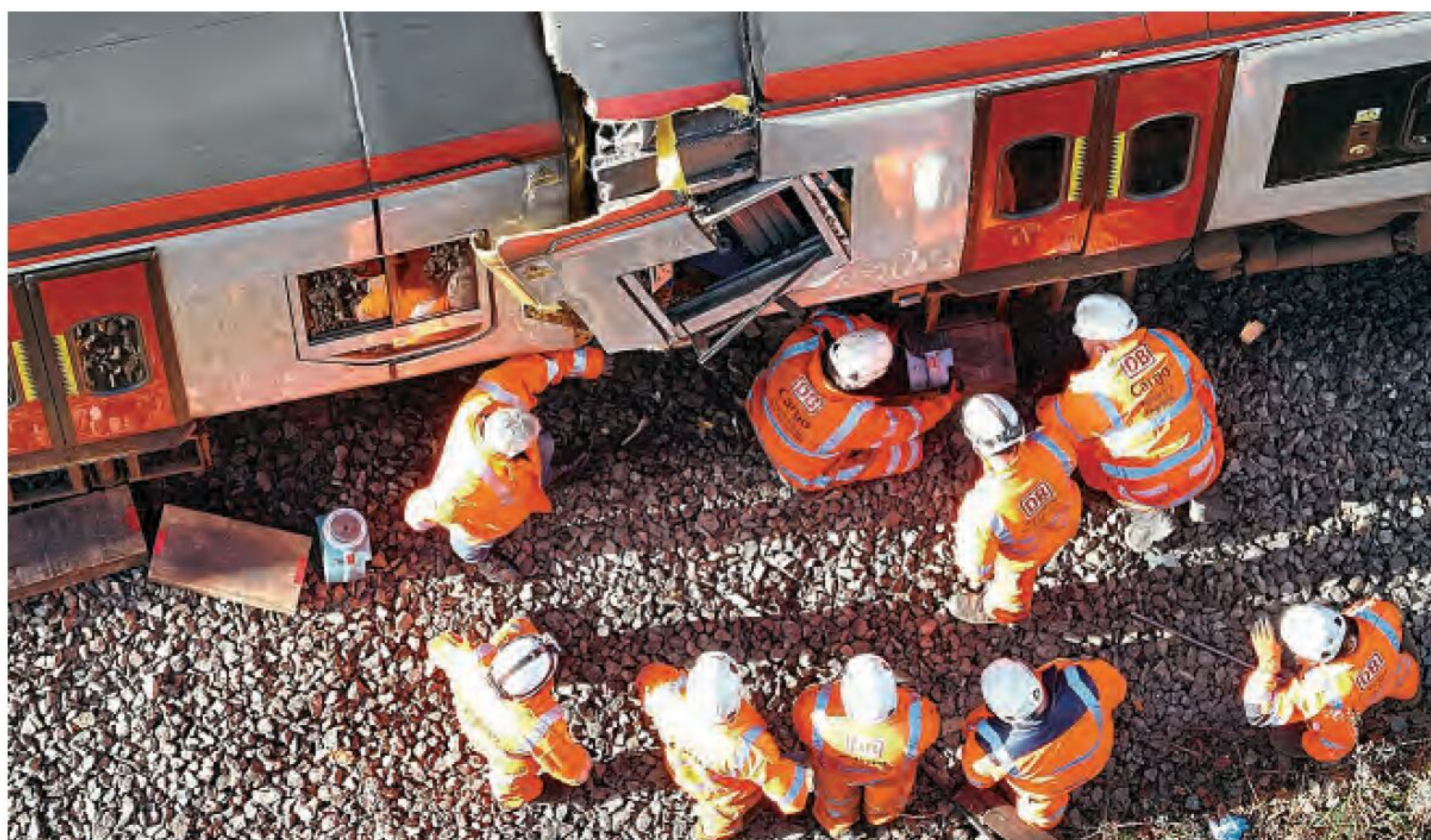
Teams work to separate the damaged Class 158 units after they collided near Talerddig loop on October 21. NETWORK RAIL
