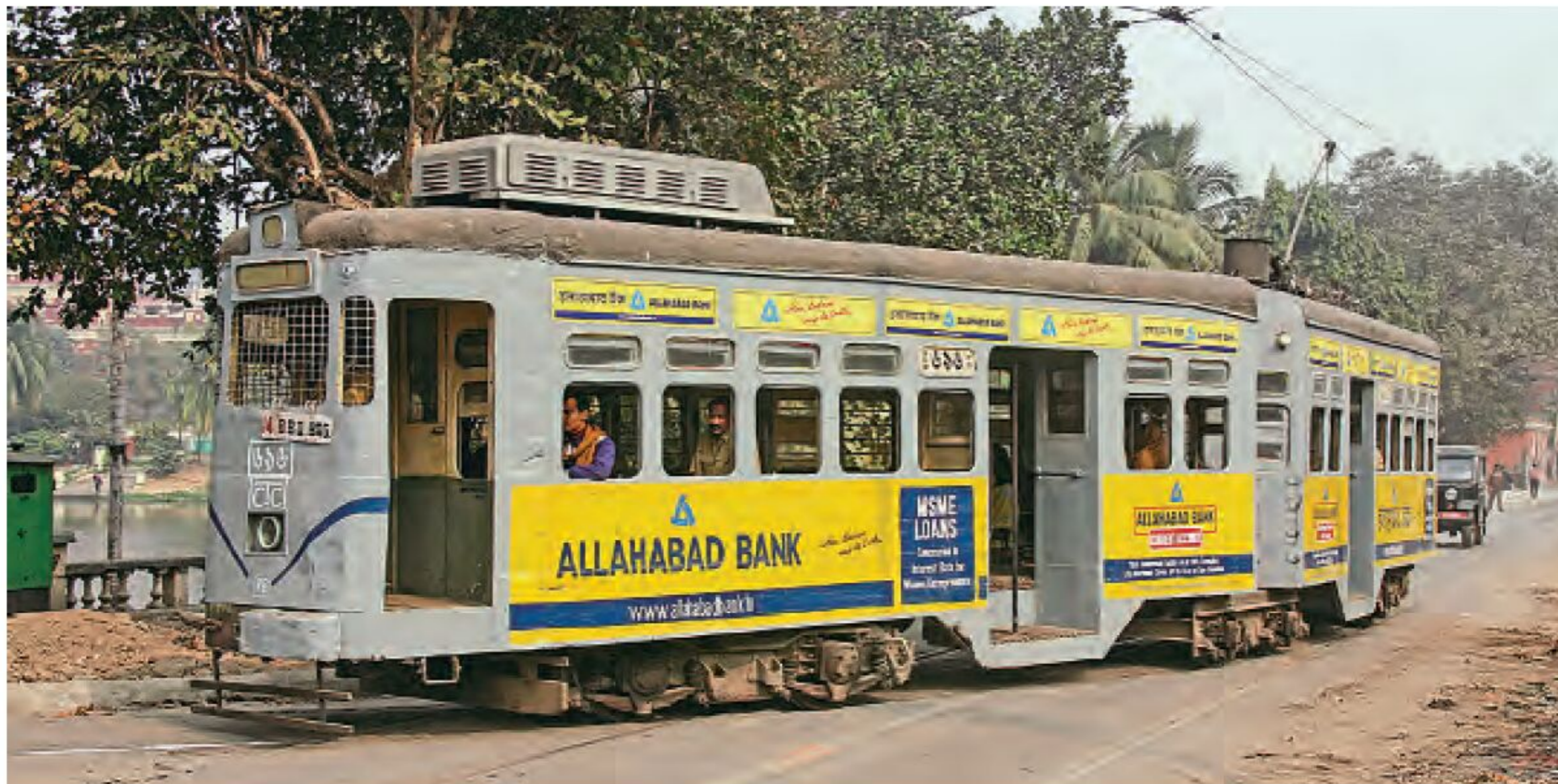
Articulated SLC Type Kolkata tram, manufactured in the city by the tram company at its Nonapukur Works, seen in the central BBD Bagh area of the city on January 31, 2011. Trams no longer run on this section of the network. MARK TORKINGTON
