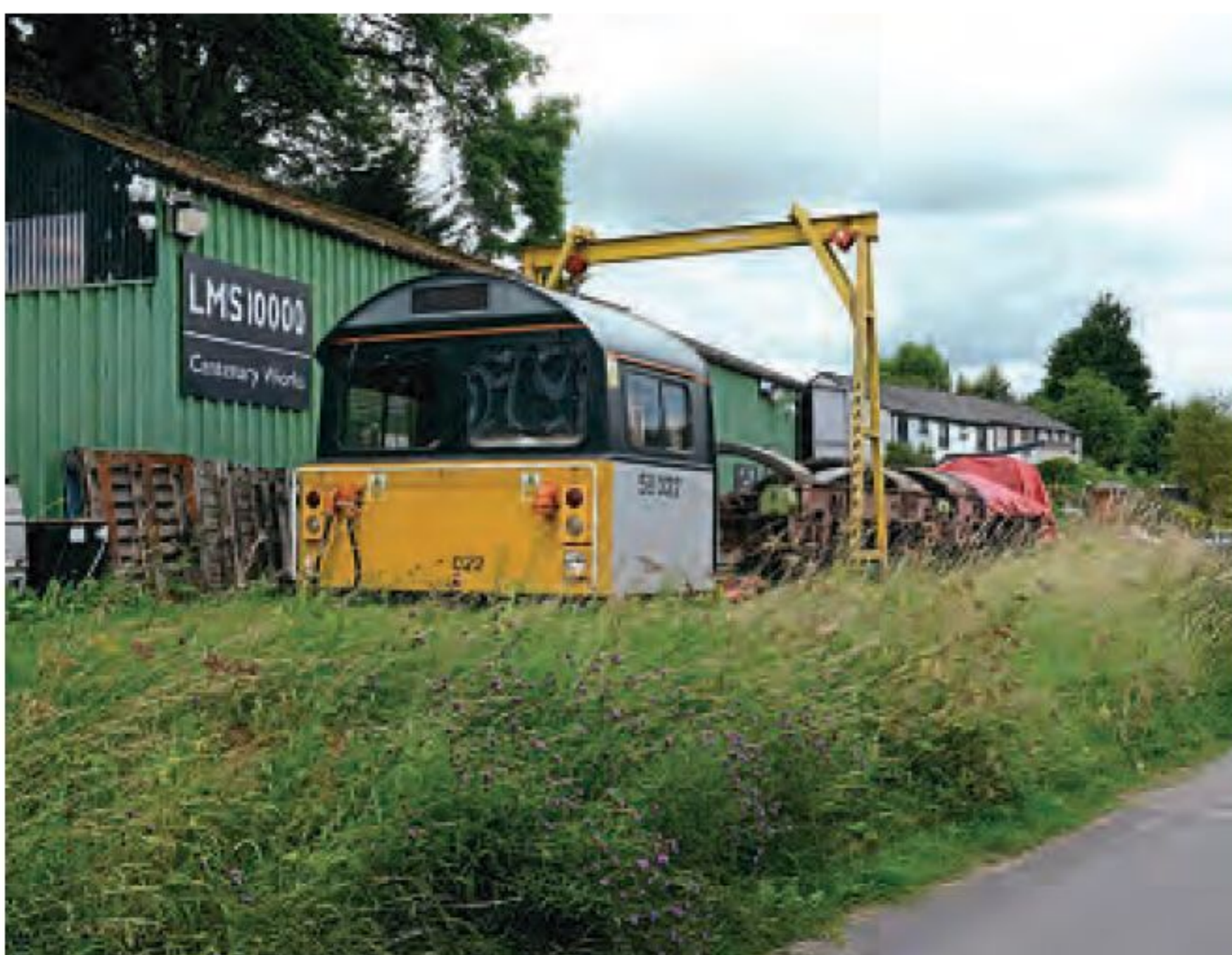
The IDRS's 'Centenary Works' at Wirksworth, Ecclesbourne Valley Railway, on July 26, with one of the cabs from donor loco No. 58022, and behind that the EM2 bogies that will be used in the new build.
