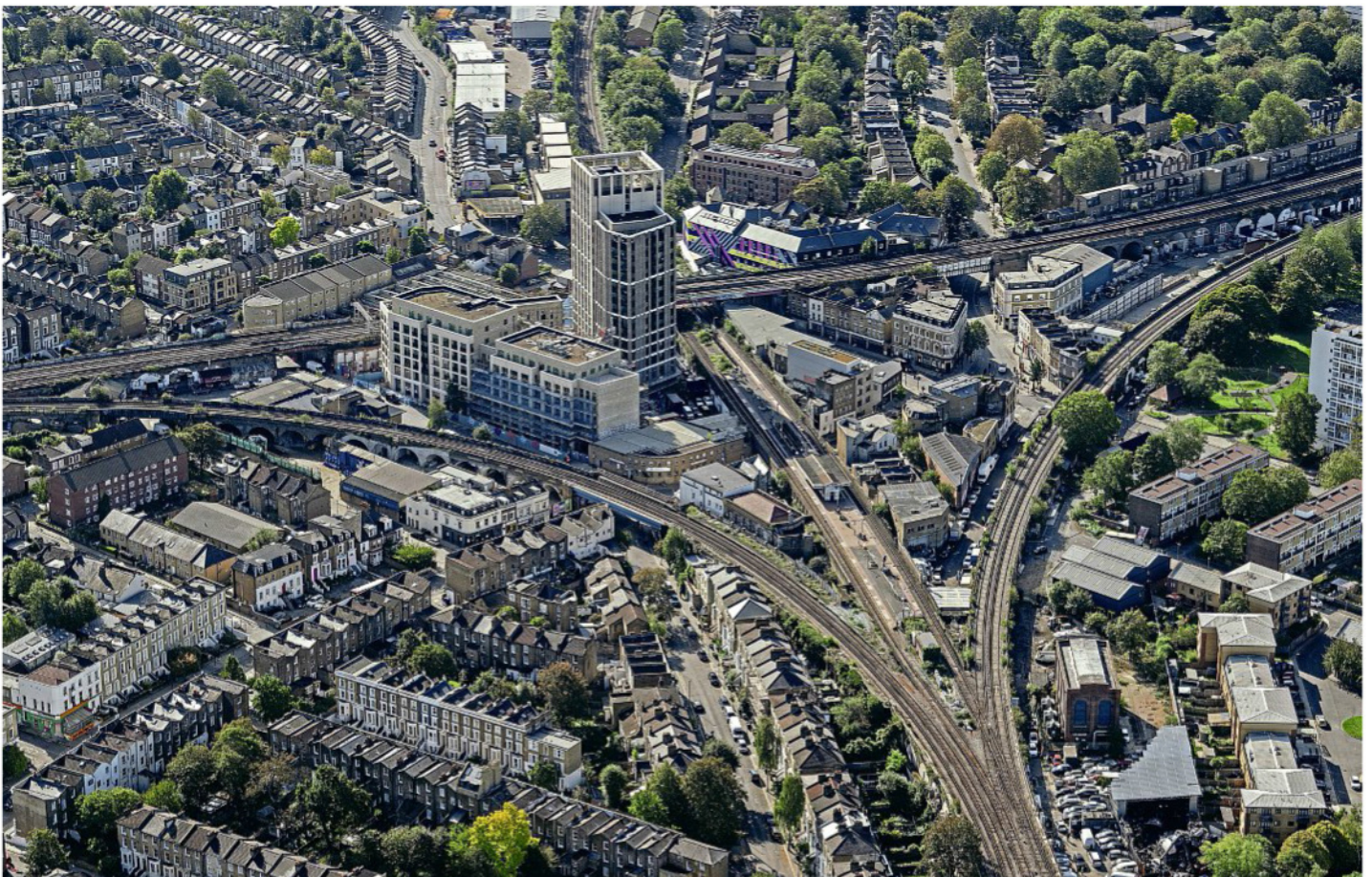
South of Waterloo, but on the line from Blackfriars, is Loughborough Junction. This view, looking south, shows the two curves that connect east and west to the South London Line through Denmark Hill, but only the Blackfriars line has a station here.
