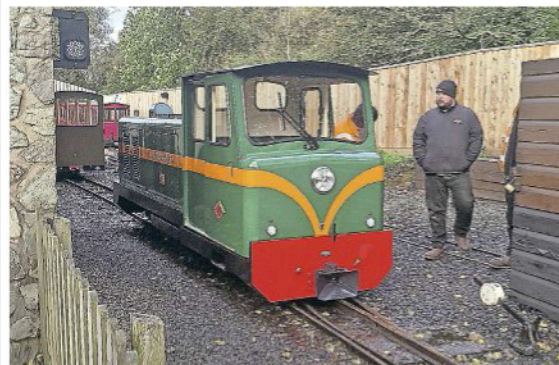
The new diesel locomotive built by Alan Keef Ltd pictured following delivery to the 15in Lappa Valley line. The loco was built to work with the new passenger train constructed by Keef's. TOM GOODMAN
