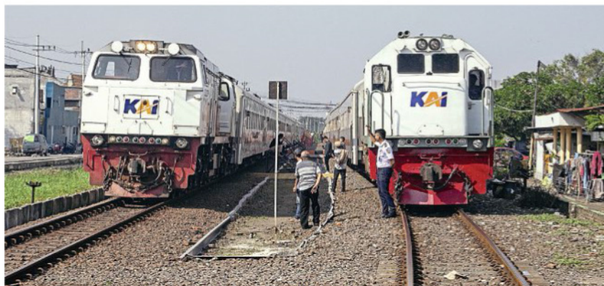
One of the oldest diesel locos in passenger service, GE U18C design No. CC201 77 05 (right), dating from 1977, waits at the small station of Gedangan on May 14 with a suburban train heading into Surabaya, while an express train from Malang headed by 2013-built GE CM20EMP design No. CC206 13 47 (left) rushes past. MARK TORKINGTON
