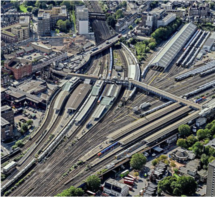
Flying west from Loughborough Junction we reach the major station at Clapham Junction. In this view looking south, the main part of the station is in the centre of the photograph with platforms for services from Victoria to the South and from Waterloo to the South West, while a long footbridge connects to the Windsor Lines platforms. In between are the station's extensive carriage sidings.
