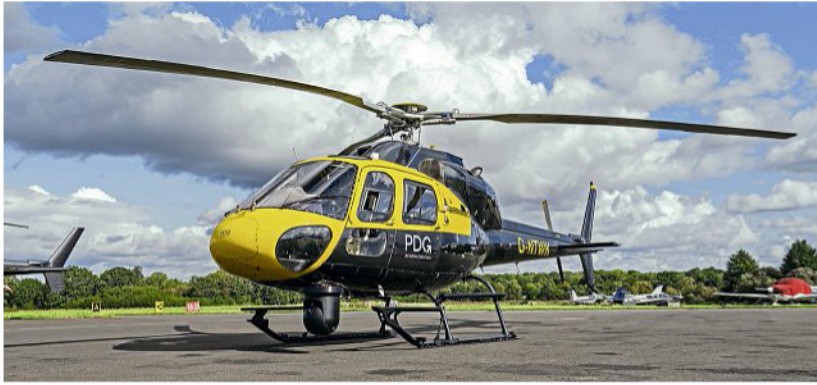
Network Rail Air Operations helicopter registration G-NTWK ready for take-off at Elstree Airfield. It is a French-built Eurocopter AS355 Twin Squirrel leased from PDG Helicopters. Note the imaging equipment attached to the underside of the fuselage.
