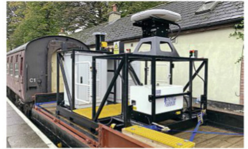
ABOVE: The wagon within the train carrying apparatus including satellite and generator equipment.
