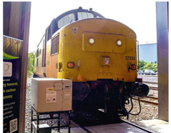
Colas Type 3 No. 37254 connected to a solid fuel oxide cell system during the demonstration at the company's Rugby depot on September 21. HOPE DREW/ADELAN LTD
