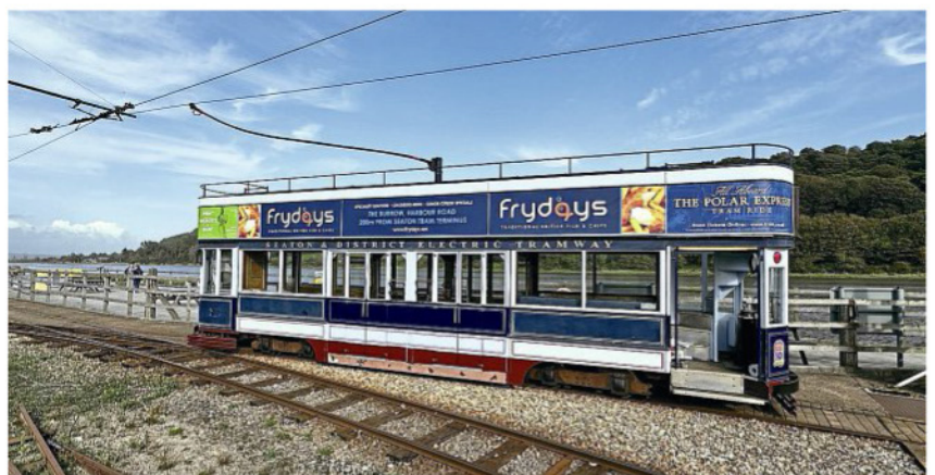
With its central section now fully enclosed with doors, Seaton Tramway No. 9 is seen at Riverside depot. SEATON TRAMWAY
