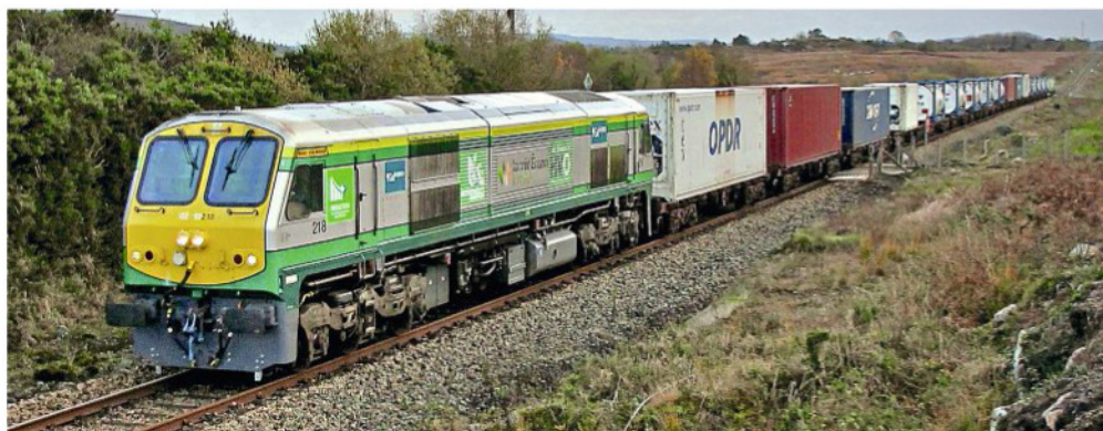
VEG-POWER ALLOWS CARBON NEUTRAL FREIGHT: 201 Class loco No. 218 is undergoing trials to use Hydrotreated Vegetable Oil (HVO) instead of diesel fuel as part of Iarnród Éireann's strategy to become carbon zero. On November 7 it worked its first freight services since conversion and is seen north of Foxford on the Ballina branch working the Dublin North Wall to Ballina liner. NOEL ENRIGHT
