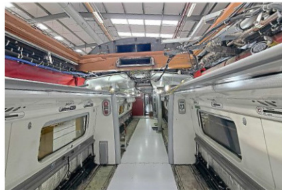
A view inside the stripped-out shop – the roof has to be removed as it is the best way to move equipment in and out.
