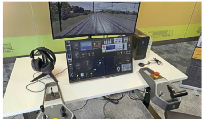
Right: A close-up of a 'light' simulator, with screens showing the route ahead and in-cab equipment, plus controls for brakes (left) and power (right).
