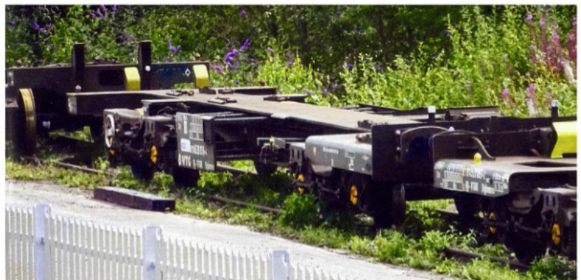
FWA 'Ecofret' flat No. 83 70 4520 016-4 was one of many such wagons stored in Cockshute Sidings, Stoke, on August 11.
