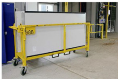
Above: Replacement floorboards arrive as sets in these 'toast racks', one for each carriage, although replacement depends on condition of the originals.
