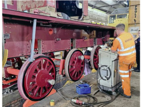
Newstead being rewheeled at Tunbridge Wells West shed on October 1. SPA VALLEY RAILWAY
