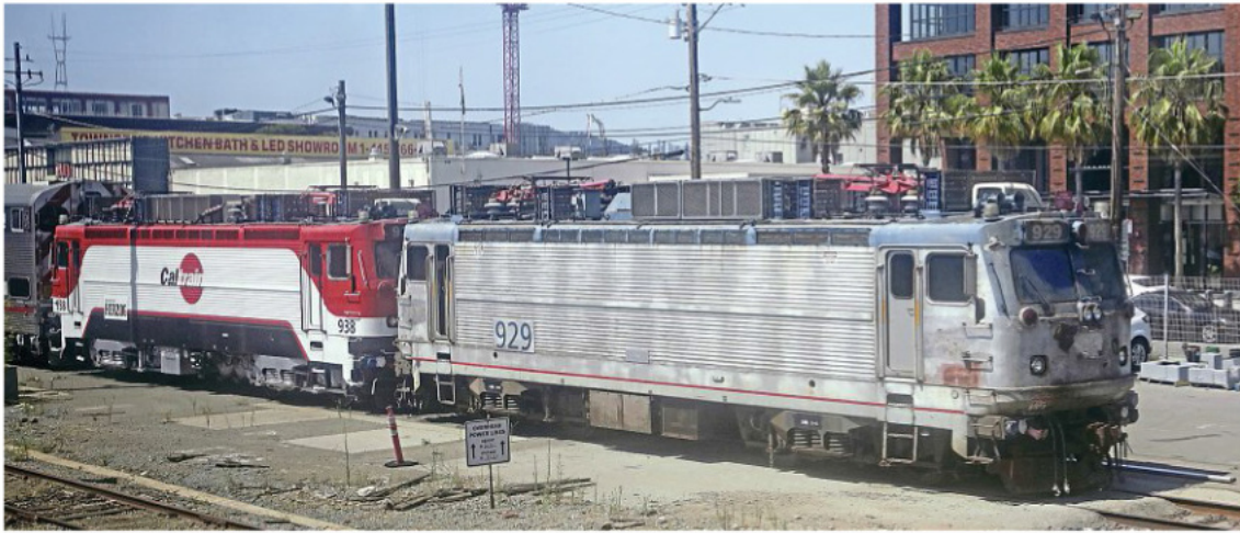
Ex-Amtrak Class AEM7 electric locos Nos. 929 and 938 (in 'Caltrain' livery) in the yard at San Francisco 4th Street station on August 23. The locos will be used for test trains on the newly electrified line. KEITH FENDER
