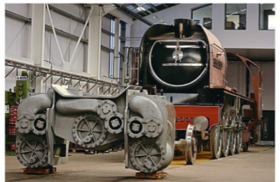
The new monobloc cylinder is seen in front of 'P2' No. 2007 Prince of Wales on Saturday, October 14, in the Trust's Darlington works. A1SLT
