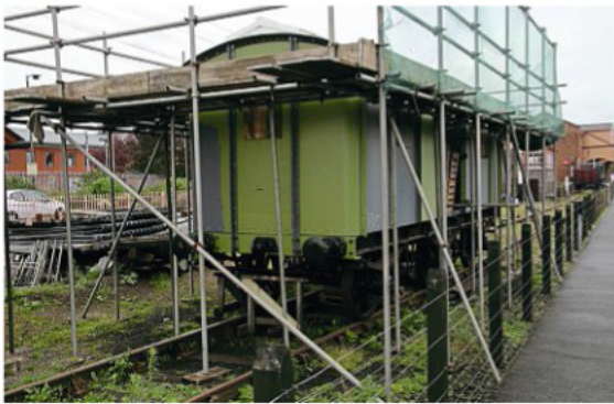
GWR No. 14984 is an iron-bodied, six-wheeled workshop van built for the GWR Signal Department. It is seen undergoing restoration at Kidderminster Railway Museum on October 5. GARETH EVANS
