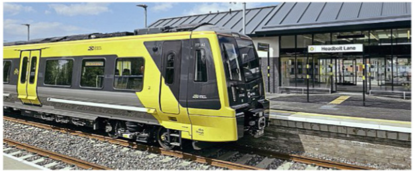
Running on battery power, Stadler Class 777 No. 777152 sits at the new Headbolt Lane station on October 5.
