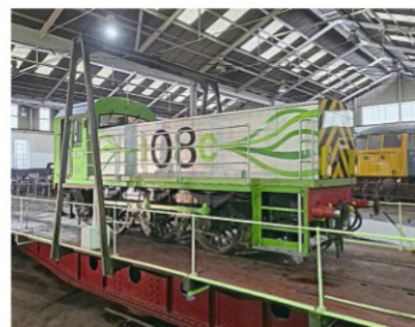
The battery compartment is much lower than the former diesel engine compartment, allowing a much improved view over front section. There are also new LED lighting clusters at both ends.
