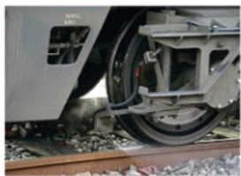
The on-board spraying equipment in action. PAUL BICKERDYKE
