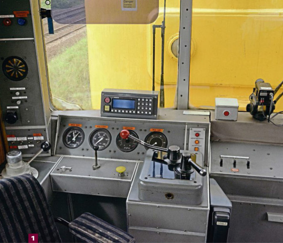
1: The driving controls at No. 2 end. There is a forward-facing video camera at each end (the black box on the right) with the feed going to a TV screen.
