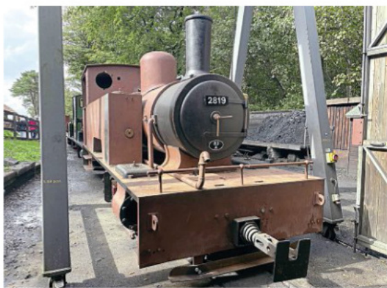
Bagnall 4-4-0T 2819/1946, previously Charles Whytock , now Sir George Newnes , pictured, with permission on September 24 from inside the loco shed at Woody Bay. The smokebox numberplate is the engine's works number as reflected by its owning group, while the Shedcode plate 83A was Newton Abbott. Behind the Bagnall are Hunslet 0-4-0ST gala visitors Lilla and Hugh Napier . JOSH BRINSFORD
