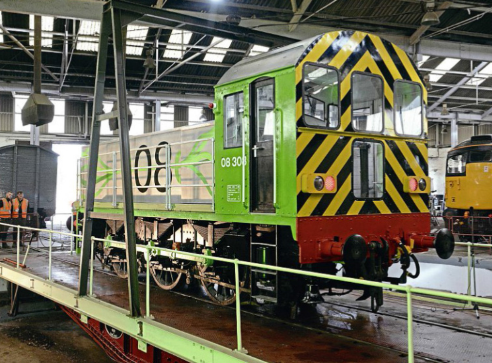
Re-engineered to run on battery power, Positive Traction's No. 08308 poses on the turntable inside Barrow Hill Roundhouse for its official launch on October 19. ALL PHOTOS BY PAUL BICKERDYKE
