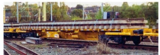
New Network Rail/Wascosa FEA-W flat No. 81 70 4524 139-2 at Bescot Yard on November 6, carrying 60ft track panels. S F LAPPAGE
