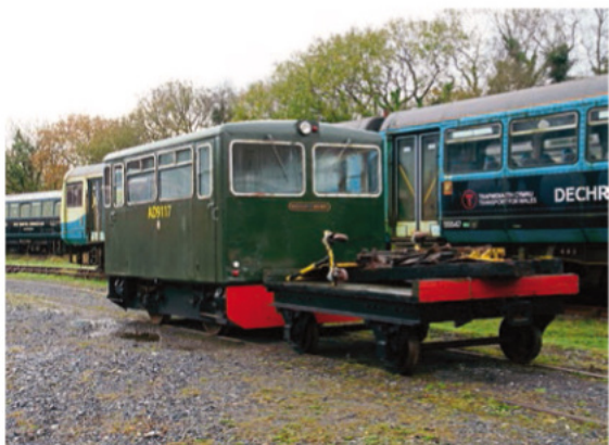
Baguley-Drewry railcar No. AD9117 and its flatbed trailer is seen at the Llanelli & Mynydd Mawr Railway, Cynheidre. In full working order and available for use by the permanent way department, it will be supporting the winter maintenance programme. DAVID MEE
