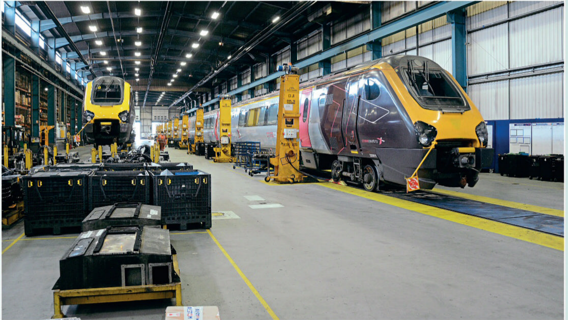
Above: The main two-road maintenance shed has two different types of jacks that can raise a complete 'Voyager' in one go. CrossCountry's five-car No. 221134 is to the left and four-car No. 220011 to the right.
