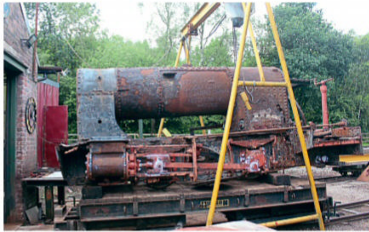
AS reported last month, ex-Renishaw Sugar Estates Avonside 0-4-0T 1986/1926 Renishaw No. 2 is now at Apedale Valley Light Railway following its purchase by a Moseley Railway Trust member. Pictured on July 10 the message chalked on the boiler says, "For Sale. Good cond[ition] One Granny owner Needs new whistle"! Subsequent stripping down included lifting the boiler on July 24. One encouraging discovery is that the wheels are in surprisingly good condition and look as if new tyres were fitted shortly before the loco was withdrawn. PETER NICHOLSON
