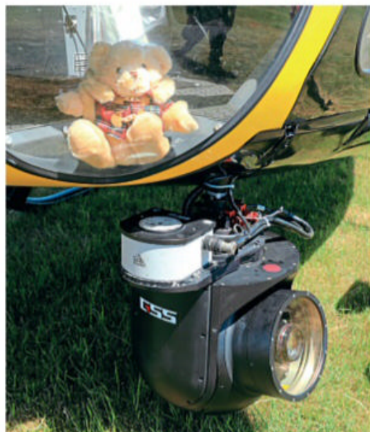
High-resolution images on the National helicopter are captured by this Canon 1DX Mk.3 camera with 85mm. PHIL MARSH
