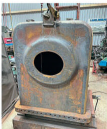
The new inner firebox for the Cavan & Leitrim Railway's 0-4-2T Dromad . C&LR
