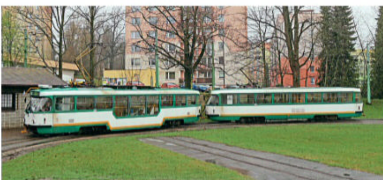
Services to Jablonec were operated by modernised Tatra T3 vehicles and it is likely these will be regauged to 1435mm and retained for use once the line reopens. T3R PLF part low floor car No. 28 leads high floor T3R PV No. 40 at the Jablonec nad Nisou terminus on April 7, 2017. KEITH FENDER
