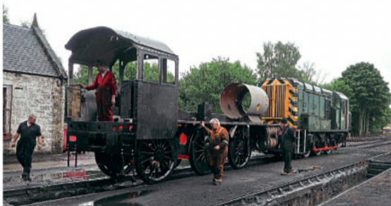
No. 46464 is shunted by Class 08 No. D3605 into Aviemore shed after rewheeling on July 28. IAIN SMITH
