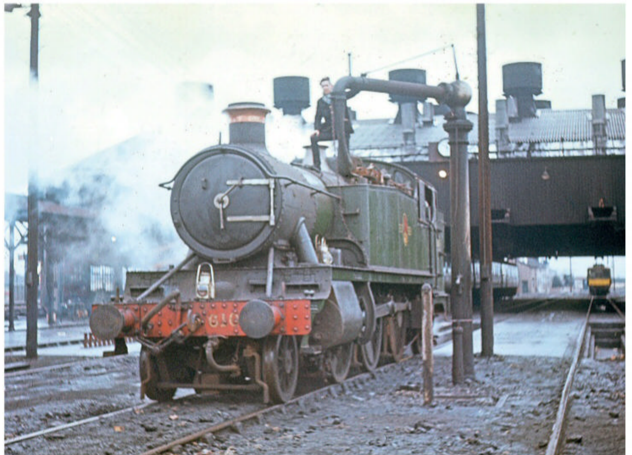
2-6-2T 'Large Prairie' No. 6106 about to leave Southall for Taplow on March 26, 1966 – Jon Barlow on top of the tank filling it with water. GWS
