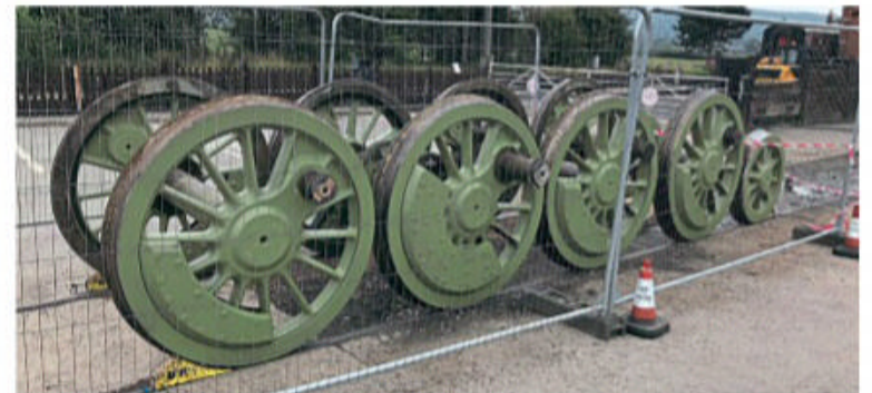
The wheelsets have been refurbished – including retired, crank pins reground and journals polished by South Devon Railway Engineering. They have been painted and are now ready for fitting. 2874 TRUST
