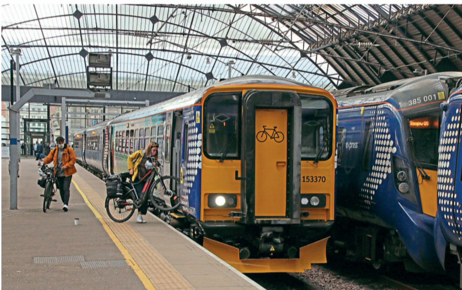
SCOTRAIL 'BIKE TRAIN' IN TRAFFIC: No. 153370 is pictured being loaded with bicycles at Glasgow Queen Street as part of the 10.34 to Oban on August 18, 2021 with No. 156457. The '153' is one of five being converted to carry up to 20 bicycles and other large luggage on ScotRail's scenic lines, the first entering traffic on July 19. IAN LOTHIAN
