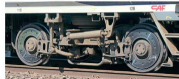
A Class 195 with the yaw damper removed. The damper bracket (arrowed) is still attached to the body, and it is the four bolts which are found to pull out of their T-channel housing in the underside of the body shell. There is no fault with the damper bracket casting, only with how it is attached to the body. TONY MILES
