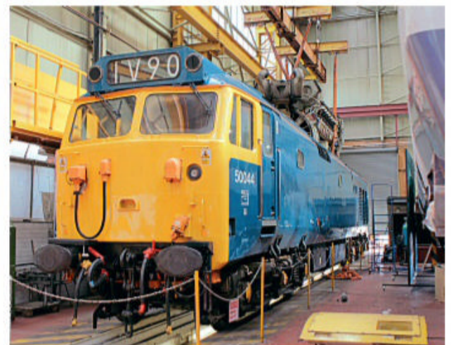
An engine lift for 50044 at Brush in 2014 showing the main generator carcass/windings. ANTHONY MIDDLETON
