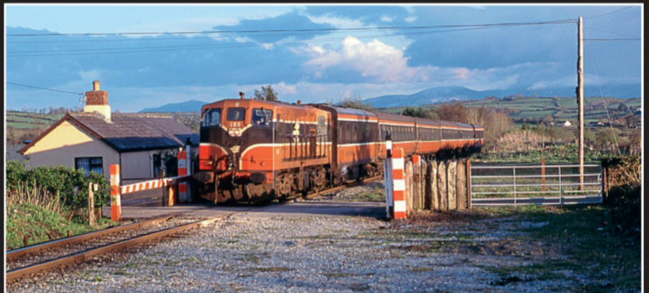
Ballybrack, situated between Killarney and Farranfore in Co. Kerry, is the location for this view of 'Baby GM' No. 165 working the 17.10 Cork to Tralee service on April 10, 1998. The train is made up of Cravens coaches in IÉ livery with a 'Dutch' generator van on either end. BARRY CARSE
