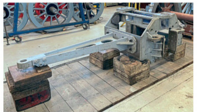
The new pony truck frame for No. 2007 Prince of Wales at Darlington Locomotive Works. A1SLT
