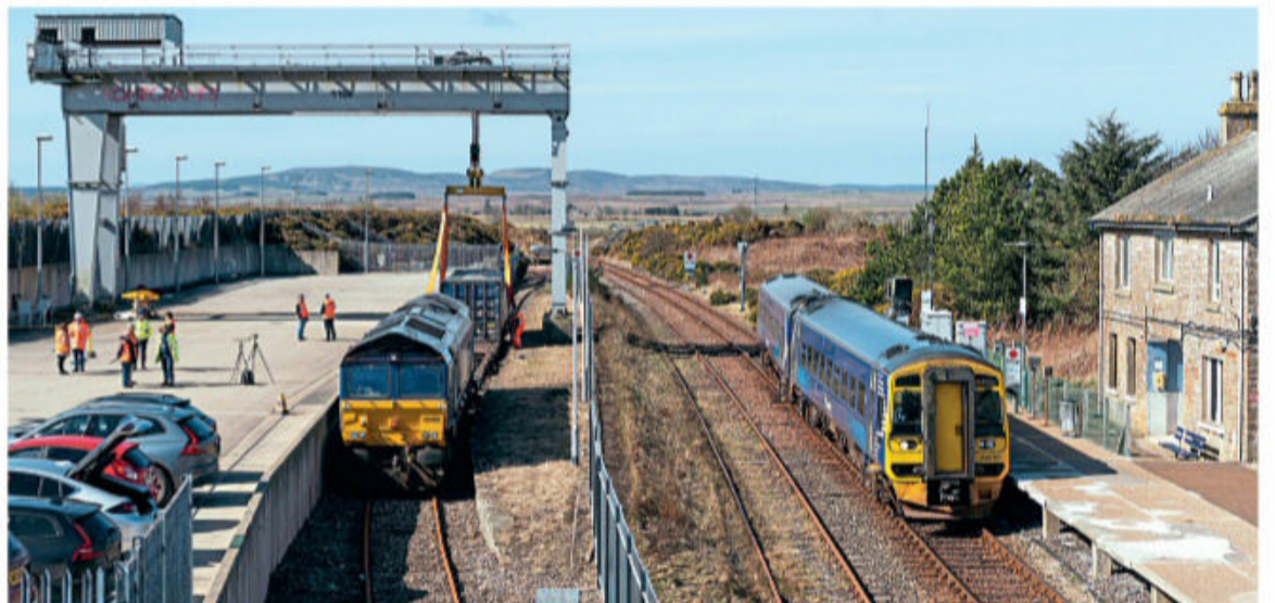
NEW FREIGHT TRIAL FOR FAR NORTH LINE: A commercial demonstration of moving intermodal containers by rail from Inverness over the Far North Line to Georgemas Jct took place on April 22. DRS Class 66 No. 66302 hauled a pair of IKA flat wagons and one Tesco curtain-sided container the 147 miles to Gerogemas to check the unloading and loading facilities normally used for nuclear waste from Dounreay. The purpose was to check the crane's suitability for possible future traffic. PICTURE: NIAL LAYBOURNE
