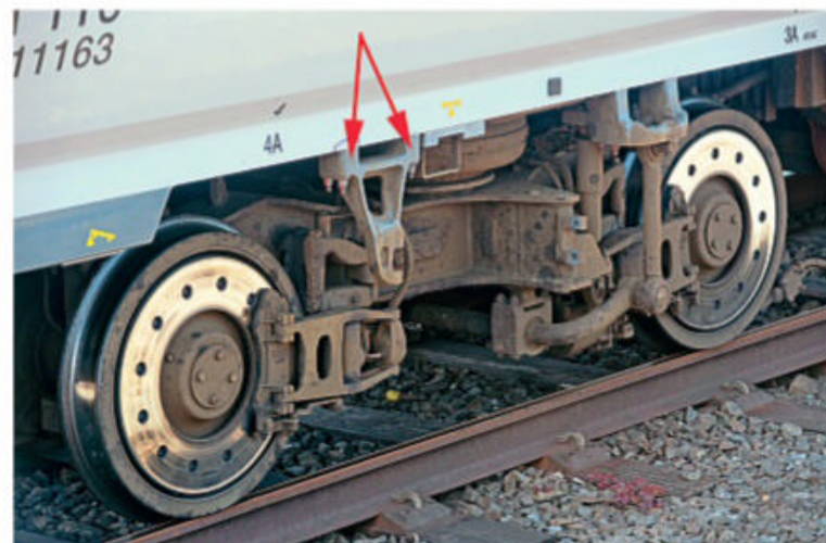
A Class 195 with the yaw damper removed. The damper bracket (arrowed) is still attached to the body, and it is the four bolts which are found to pull out of their T-channel housing in the underside of the body shell. There is no fault with the damper bracket casting, only with how it is attached to the body. TONY MILES
