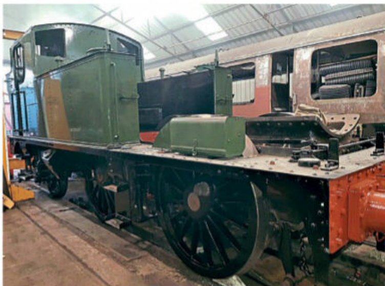
Re-wheeled '14XX' No. 1466 stands in the workshops of Western Steam Engineering as the overhaul turns to focus on the boiler. ED FREEMAN/WSE
