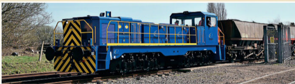
The first of the new Clayton 'CBD80' hybrid shunters on test at the Chasewater Railway on March 30. ALISTAIR GRIEVE
