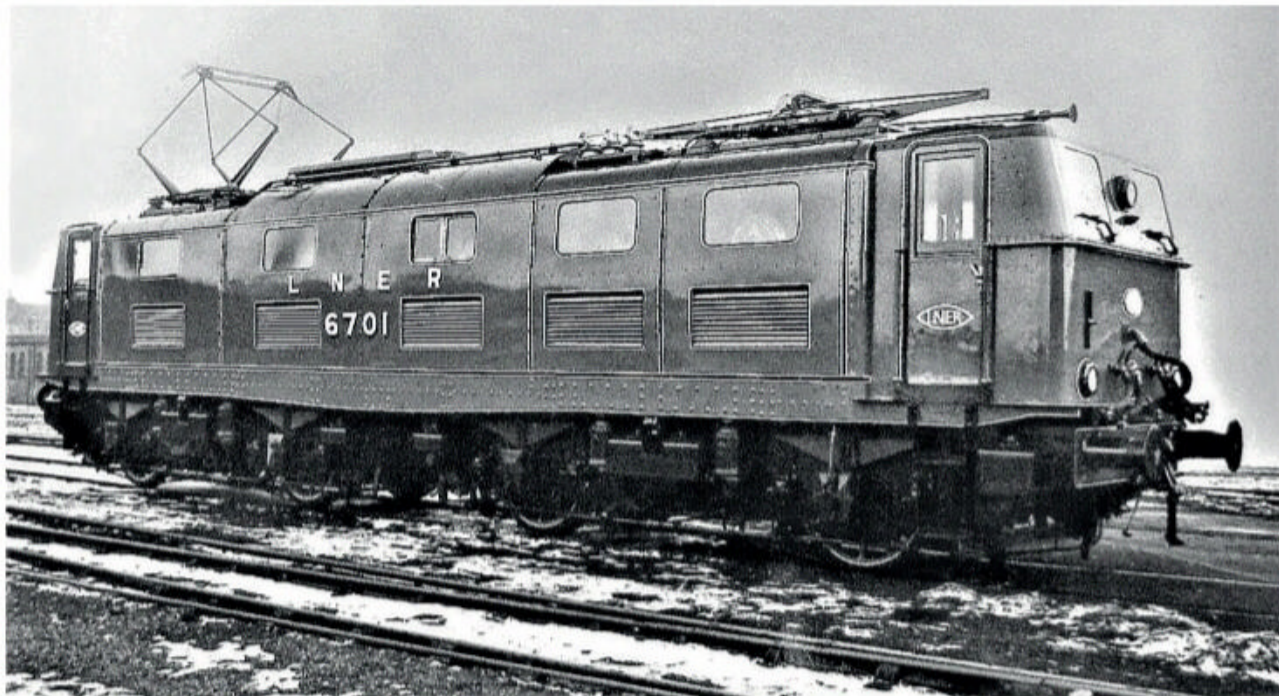
Often overlooked, Gresley's electrification programme, though held up by financial constraints during the 1920s and 1930s, promised much and took giant steps forward. This was nowhere more apparent than in the production of this prototype Bo-Bo locomotive (No. 6701) for use on the Woodhead line. Here is the completed loco in 1941 at Doncaster.
