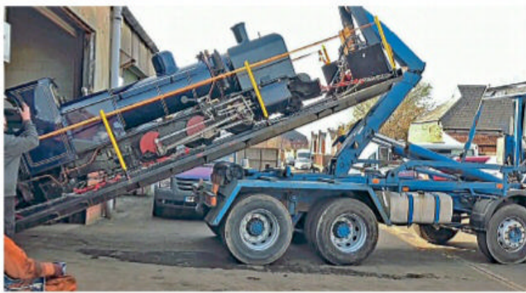
No. 6 Blickling Hall emerges from North Bay Railway Engineering Services on March 30 to return to the Bure Valley Railway following fitting of a new boiler. The loco is being loaded onto the novel transporter developed by NBRES last year (RM, November 2020). The vehicle is available for hire to heritage lines for movement of comparatively small locomotives. NORTH BAY RAILWAY ENGINEERING SERVICES
