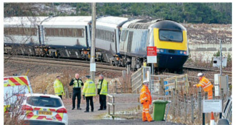
HST power car No. 43012 and a trailer vehicle derailed on the up to down crossover at Dalwhinnie. JOHN CUMMINGS
