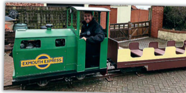
The restored Exmouth Express. The 4wDM was built by Geoffrey Kichenside in 1978 using one end of Shepperton Metal Products 2-4w-2DM Meteor III of 1969. This followed accident damage to the original loco. The other end now forms part of Midget, which was at Hatfield House Farm Railway, Hertfordshire, until closure in 2018. PICTURE COURTESY EXMOUTH MINIATURE RAILWAY
