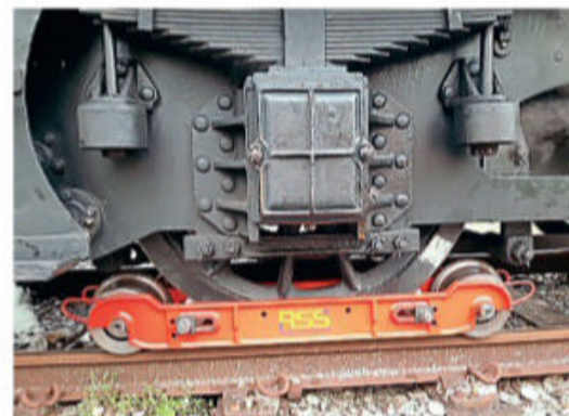
The WheelSkate employed to lift the tender wheelset clear of the rail and enable the 'Black Five' to be moved following its failure. ANDREW GOODMAN/RSS
