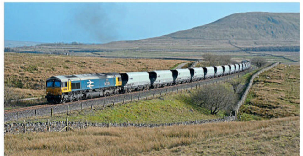
Colas Railfreight Class 56 No.56302 Peco climbs past the site of the former military sidings at Tors Road Bridge, Okehampton, with the 6F27 14.36 Westbury to Crediton on April 18; one of two trains delivering 5,000 new concrete sleepers for the Okehampton line relaying in connection with the reopening the line to passengers. The Class 56 is due to remain on the line to act as a 'Super Shunter' for the track relaying work. RUSSELL AYRE
