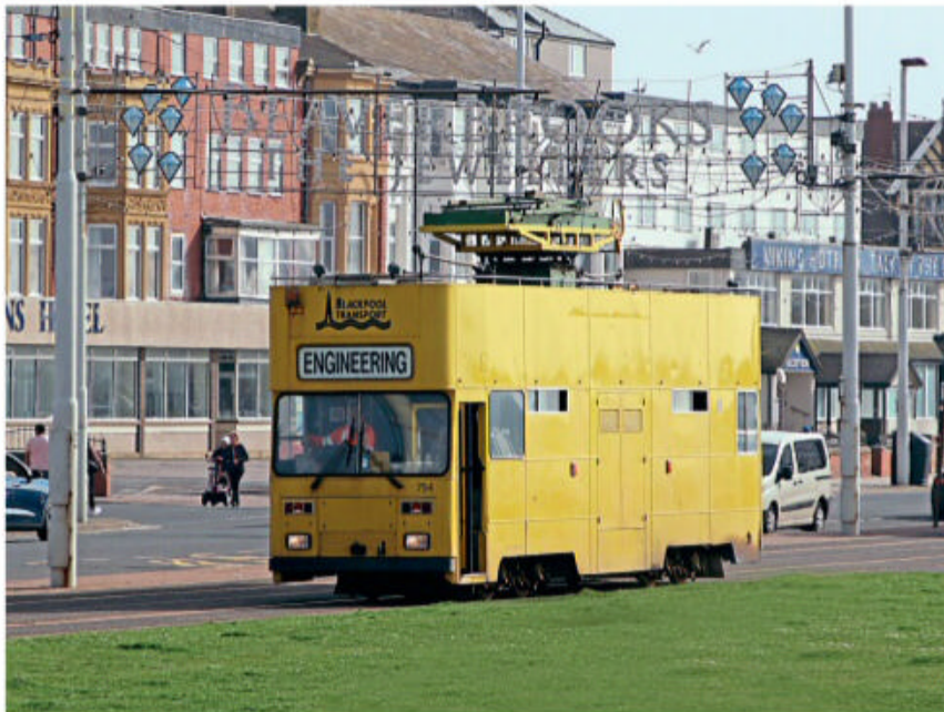
BLACKPOOL'S DIESEL TRAM: Engineering car No. 754 was spotted in action on the Blackpool Tramway on March 30, slotting in between the service of 'Flexity' trams. No. 754 has been based in the Lancashire town since 1992, replacing the earlier fire-damaged No. 753. It features a roof-level inspection gantry and has a diesel bus engine, allowing it to run when the overhead power is turned off. It is pictured at Waterloo Road. KEITH FENDER
