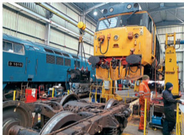
Inside the Kidderminster diesel depot, No. 50049 has a traction motor changed - one of the tasks the depot was designed for. JAMES GREGORY
