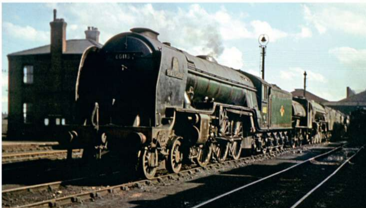
Gresley's first 'A1' built in 1922, No. 4470 Great Northern , was rebuilt under Thompson, a project which included new frames. As 'A1/1' No. 60113 in BR stock, the loco, with its 'wing' type smoke defectors, sits at Doncaster in September 1960. G PARRY COLLECTION/COLOUR-RAIL
