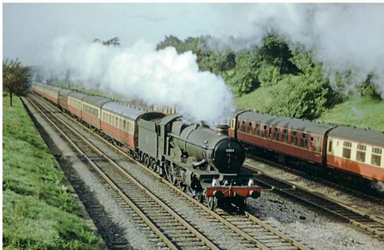
Bath Road's No. 4084 Aberystwyth Castle is less than a month out of Swindon Works after overhaul but is already showing signs of a heavy work load, with a layer of grime beginning to form and a short trail of steam leaking from one of its inside cylinder valves. It is captured here thundering through Twyford on October 11, 1958, with an unidentified eastbound express.
