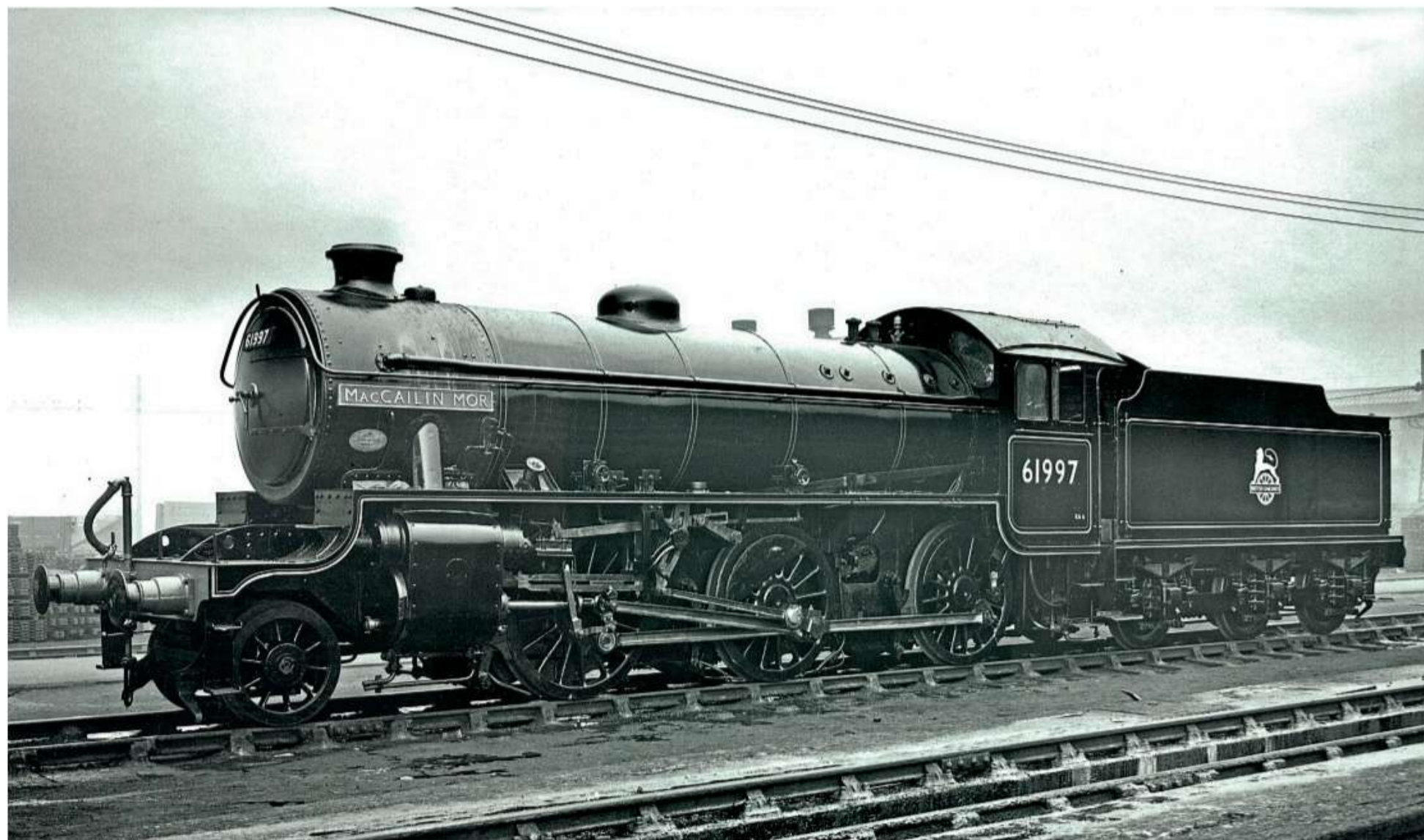
Thompson rebuilt three-cylinder Gresley 'K4' No. 3445 MacCailin Mor at Darlington in 1945 as a two-cylinder loco, with much of the work entrusted to his assistant Arthur Peppercorn. The result was a 'K1' prototype designated as a 'K1/1', and later led to 70 'K1s' being built under Peppercorn to a revised design from 1949. No. 3445 became BR No. 61997. BR DONCASTER WORKS/RM ARCHIVE
