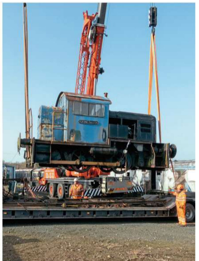
Flying Falcon flying, as Fowler 4220016 is lifted on to Pete Briddon/Heanor road transport at Meldon Quarry on March 2. Now owned by Steve Godfrey, the 0-4-ODH is not in working order and could not be shunted to where it could have been loaded by means of a ramp, hence the craneage. STEVE GODFREY
