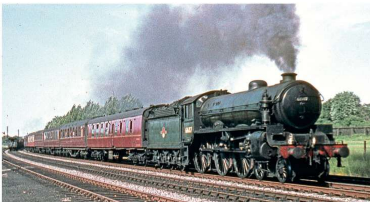
Under Thompson, 10 Gresley three-cylinder 'B17' 'Sandringhams' were rebuilt as two-cylinder 'B2s' with a 225psi boiler, North Eastern tenders and alterations to the bogie and cylinder positions. No. 61607 Blickling is seen at speed near Cambridge in May 1959. All 10 were withdrawn by the end of 1959. G D KING/COLOUR-RAIL
