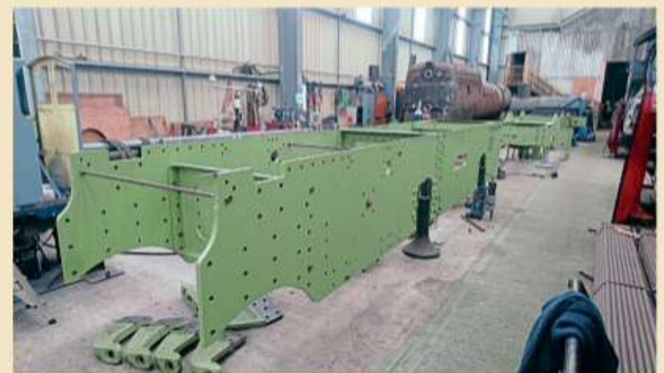
The completed main frame assembly of No. 3840 County of Montgomery at Tyseley Locomotive Works in mid-January. Fitting of the rear dragbox will follow. ALASTAIR MEANLEY
