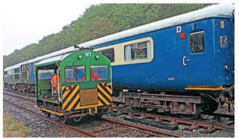
Wickham 10841 of 1975 is in operational condition on the Dartmoor Railway (DR). It is seen approaching Okehampton station from the east on August 28, 2019, carrying a permanent way gang. It was put up for sale, along with the Mk2f FO No. 3353 behind, and other items of stock. The Wickham Type 18 was refurbished by the DR track gang in winter 2014, when given the number 1. Powered by a Ford 2712E four-cylinder diesel engine, BR numbers carried were DB966033 and DX68086. On the far left is Class 31 No. 31452. PETER NICHOLSON
