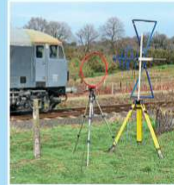
The loco undergoing electromagnetic interference tests on the Severn Valley. GBRf
