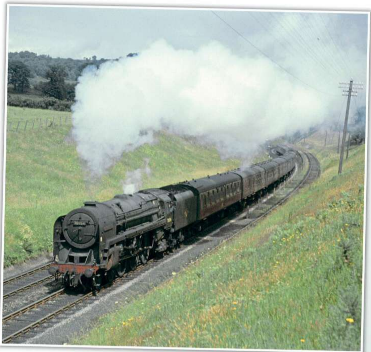
The crew on the telegraph wires doesn't seem fazed as Crewe North-based 'Britannia' No. 70054 Dornoch Firth lumbers up the bank north of Llanvihangel, Monmouthshire, with the 13-coach 9.20am Liverpool to Plymouth on July 13, 1963. The built-up (disused) siding on the east side of the cutting here gives an indication of the gradient (approximately 1-in-82) faced by locomotives approaching the station in both directions, the disused platforms just a few hundred yards away from the location of this shot, almost straddling the summit.
