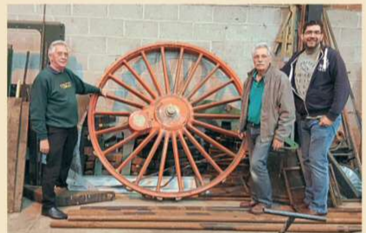
CCT trustees Richard Croucher (left), David Bradshaw and Gary Boyd-Hope with the wheel pattern for No. 3840's coupled wheels. The pattern had previously been used to cast the six drivers of No. 2999 Lady of Legend . CHURCHWARD COUNTY TRUST
