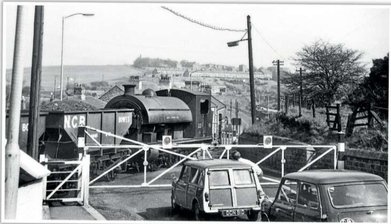
Traffic is halted on the A692 at Hobson Bank crossing to allow National Coal Board 'Austerity' 0-6-0ST No. 22 (not the same No. 22 closely associated with Springwell) to cross with a loaded eastbound train. This section of line between Burnopfield and Marley Hill had only a few months of life left when this picture was taken on April 17, 1968. The track can be seen in the middle distance curving away from the road, after which it reached Marley Hill Colliery and crossed the Tanfield Branch (now the preserved Tanfield Railway). It's hard to imagine that road once gave way to rail on this now busy stretch. TREVOR ERMEL
