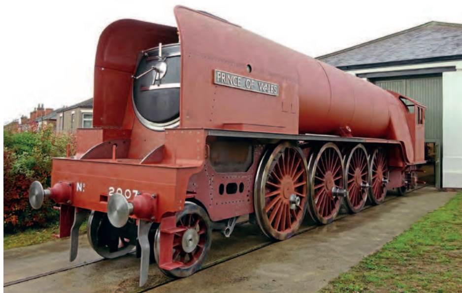
The loco outside the works offering a taster of what the massive 'P2' will look like. The boiler cladding gives a more complete appearance. A15LT
