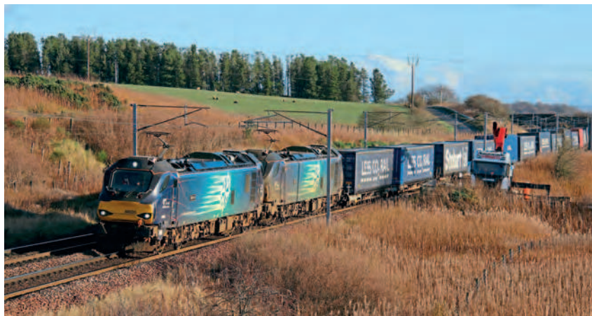
The daily Daventry to Mossend 'Tesco' train has been worked by double-headed Class 88s for some weeks now, mainly as a precaution against poor railhead conditions. No. 88005 Minerva leads No. 88009 Diana at Craighill on November 19 with the 06.24 Daventry-Mossend working. IAN LOTHIAN
