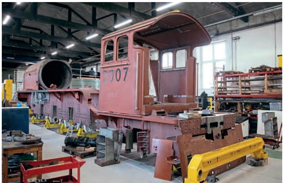
The frames, cab and smokebox inside the works at Darlington on October 7, awaiting the boiler to fill the gap. The loco’s TOPS number has been chalked on the cabside. CHRIS MILNER
