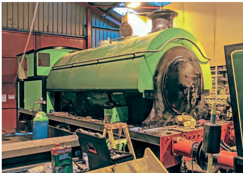
Above: Drilling underway on the smokebox of Swanscombe No. 6 to allow fitting of vacuum pipes and lubricators. MR
