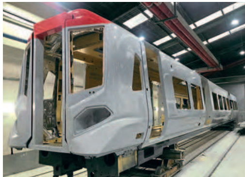
A Class 197 'Civity' bodysell on accommodation bogies at the Stadler factory in South Wales. TfW
