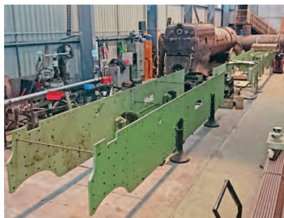
An interesting comparison between the frames of 'County' 4-4-0 County of Montgomery in the foreground, and those of Holden 'F5' 2-4-2T No. 789 behind. ALASTAIR MEANLEY
