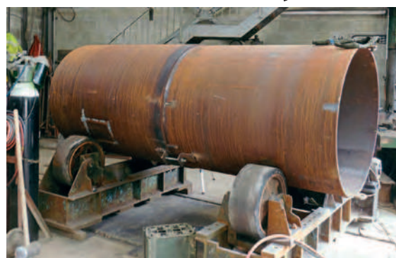
The new boiler barrel sections for the South Devon Railway's 0-4-2T No. 1420 are joined together at Buckfastleigh at the end of October last year. SDR
