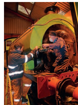
Above: Drilling underway on the smokebox of Swanscombe No. 6 to allow fitting of vacuum pipes and lubricators. MR
