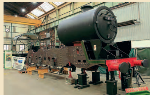
'Clan' No. 72010 Hengist as CTL Seal's works following the trial fitting of the smokebox, cab and front end during late November.
