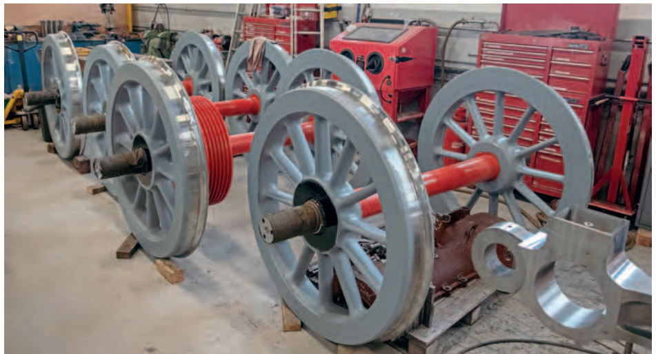
The tender wheelsets: Second from the right carries the pulley to drive the alternator. CHRIS MILNER
