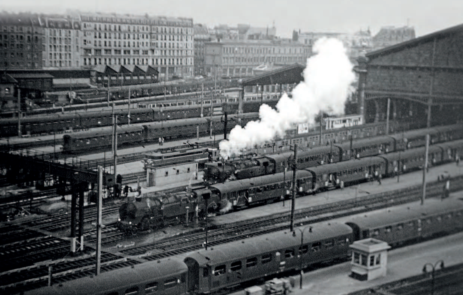
In March 1969, the commuter services from Paris's Gare du Nord to Ermont-Eaubonne and Persan-Beaumont were worked by two-cylinder SNCF Class 141TC 2-8-2 tank engines, based at Joncherolles depot. In this panoramic view, taken from an apartment overlooking the station on March 27, 1969, one of the class departs in fading light at the end of the evening rush hour. ALL PICTURES PHILIP HORTON UNLESS STATED.
