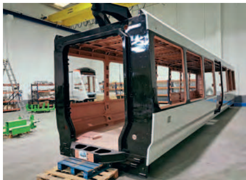
One of the tram-train cars for the South Wales Metro in the Stadler workshops. TfW
