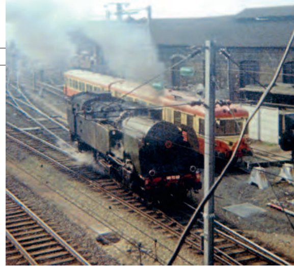
SNCF 2-8-2 tank No. 141TC 62 comes off the shed at Persan-Beaumont before working a train to Paris Gare du Nord. An SNCF two-car diesel railcar can be seen to the right. SUE HORTON
