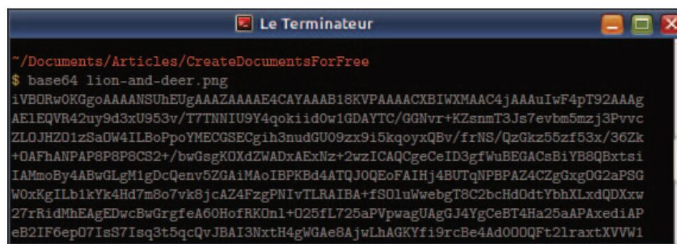
Figure 4: A text-encoded image is a huge chunk of unintelligible but plain text
