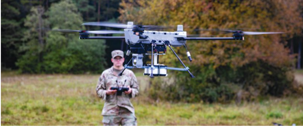
A soldier tests a 3D-printed munition dropper during Exercise Combined Resolve 26-1 in Hohenfels, Germany.
