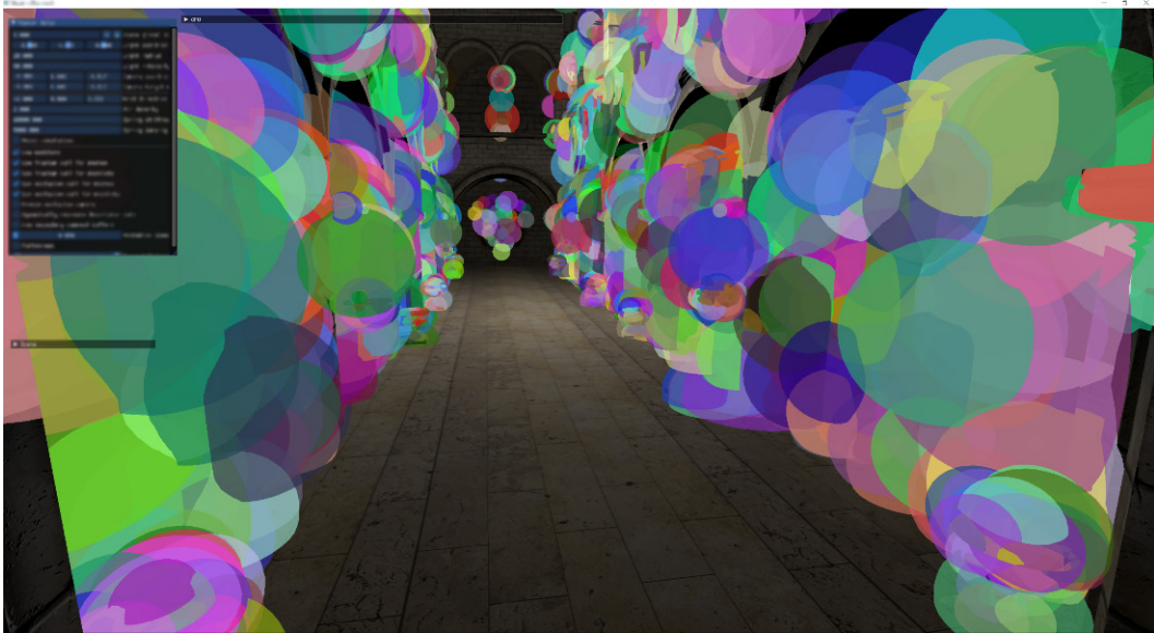
Figure 6.2 – A meshlet bounding spheres example; some of the larger spheres have been hidden for clarity
