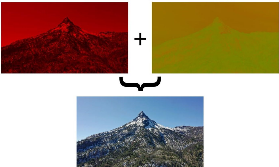
Figure 16-6. Intermediate textures showing luminance and chrominance values during YUV to RGB conversion
