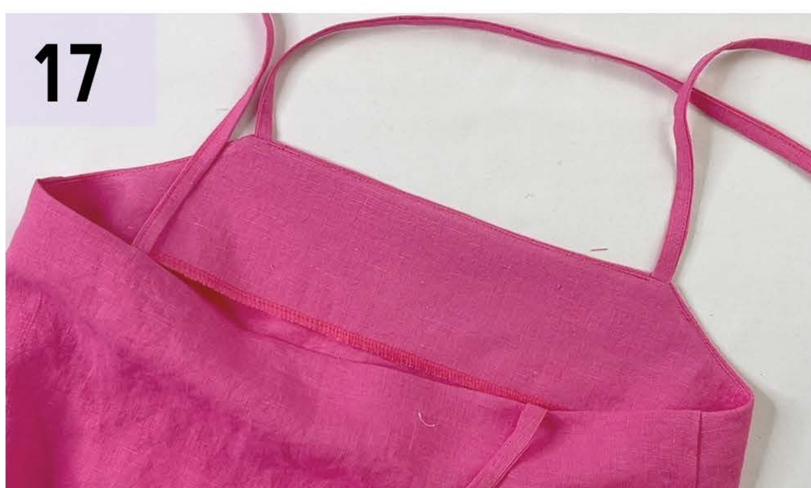
17 Turn the Facing to the wrong side and press the neckline edge.
