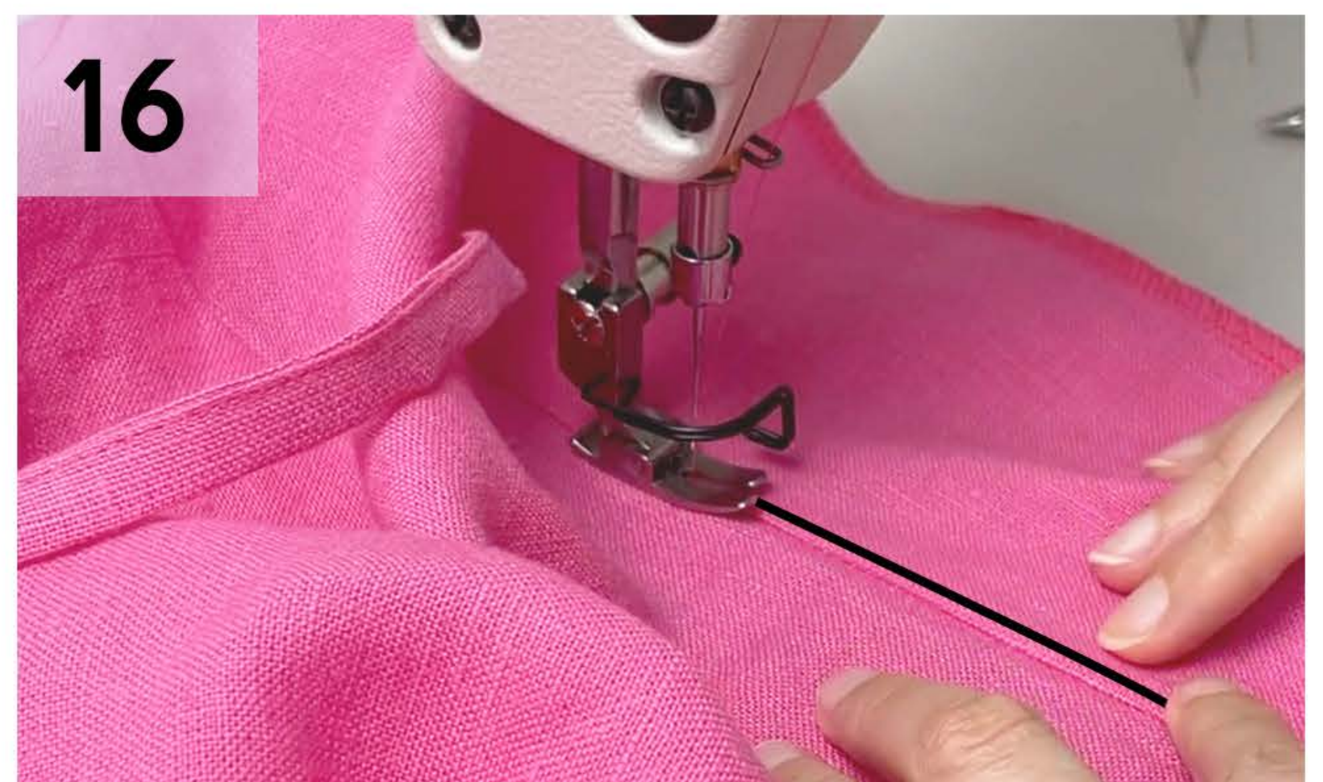
16 Turn the Facing to the right side, with the seam allowances towards the Facing and understitch the Facing 1-2 mm (1/8") from the edge, stopping before the corners and continuing after the corner.
