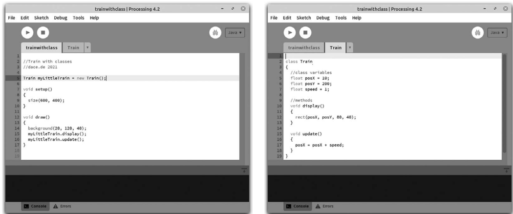
FIGURE 25.1 Typical (and recommended) use of tabs in the Processing IDE: One tab for the main program (left) and another for the Train class (right)
