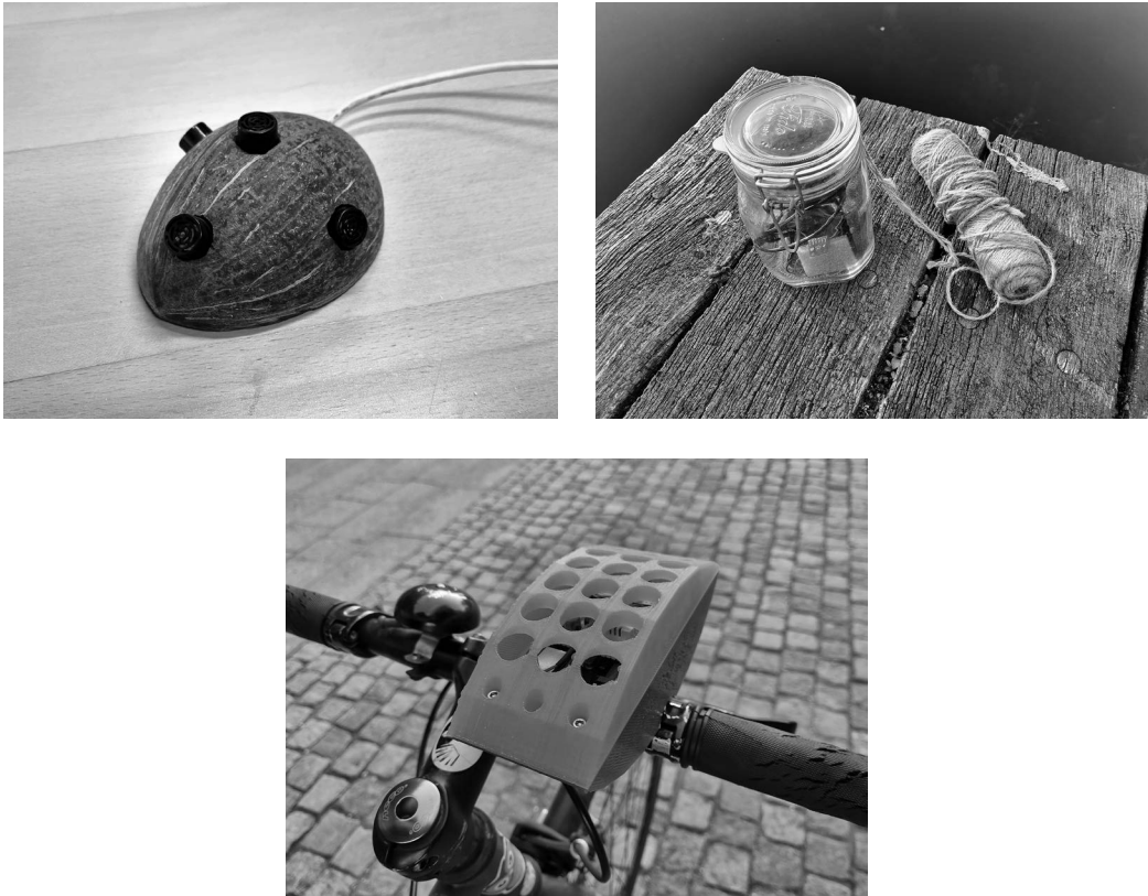
FIGURE 0.3 More Arduino projects: A mobile phone theremin, a wave measuring device, and an air quality sensor (photos by the author)
