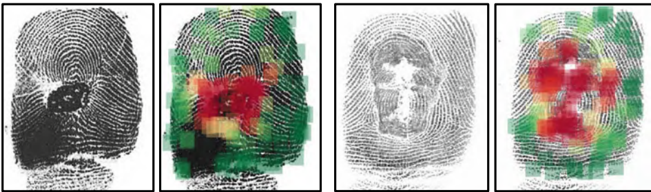
Fig. 9.16 Examples of altered fingerprint detection and localization. Local regions highlighted in red represent the altered portion of the fingerprint, whereas regions highlighted in green reflect the bonafide friction ridge area. © IEEE. Reprinted, with permission, from Tabassi et al. (2018)
