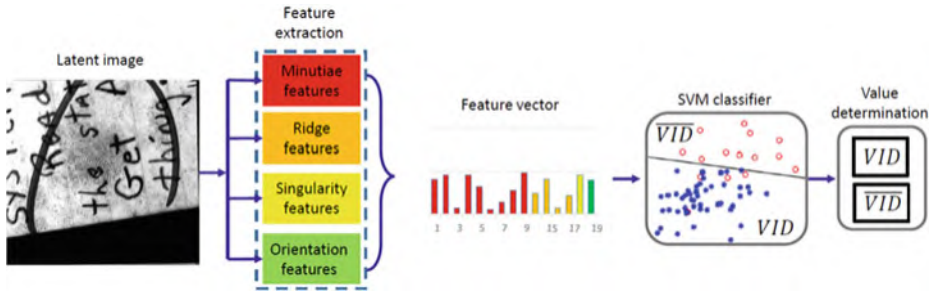
Fig. 6.29 Automatic latent value determination algorithm in Cao et al. (2016). © IEEE. Reprinted, with permission, from Cao et al. (2016)
