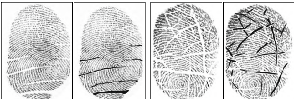
Fig. 3.48 Two examples of crease detection (in black) by Wu et al. (2003) approach. © IEEE. Reprinted, with permission, from Wu et al. (2003)
