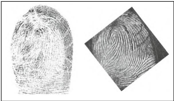
Fig. 2.15 (Left) the FTIR image of a finger whose epidermis was voluntarily erased by one hour of sandpaper rubbing and (Right) the finger in the same condition acquired with an OCT device. Image courtesy of Christophe Champod—University of Lausanne
