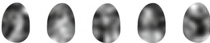
Fig. 7.13 Some examples of synthesized frequency images (Cappelli et al., 2000): light blocks denote higher frequencies
