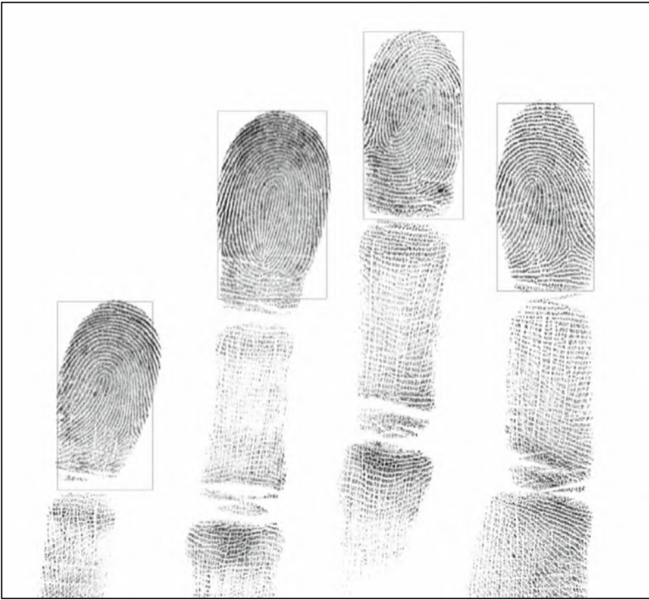
Fig. 2.25 An example of 500 dpi image ( 1558 \times 1691 pixels) acquired with the multi-finger scanner Papillon DS-30; the four rectangles show the position of the four fingerprints as located by an automatic slap segmentation algorithm
