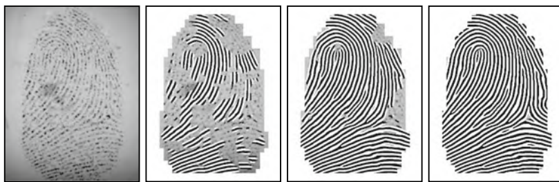
Fig. 3.46 Iterative enhancement of a fingerprint image as proposed by Cappelli et al. (2012). © IEEE. Reprinted, with permission, from Cappelli et al. (2012)
