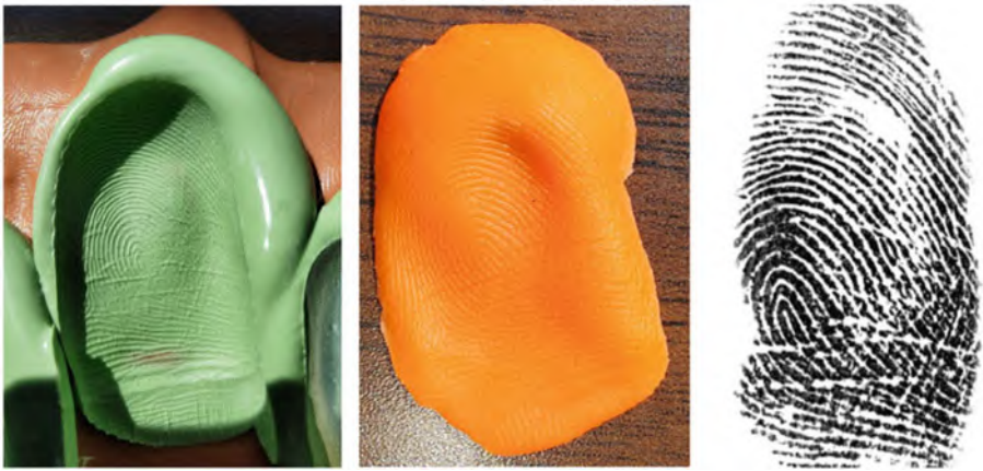
Fig. 9.10 An example of cooperative fabrication where the mold (left side) is made of dental material and the spoofer (central image) of PlayDoh. On the right, a fingerprint image produced by the spoofer. Image courtesy of Stephanie Schuckers and David A. Yambay
