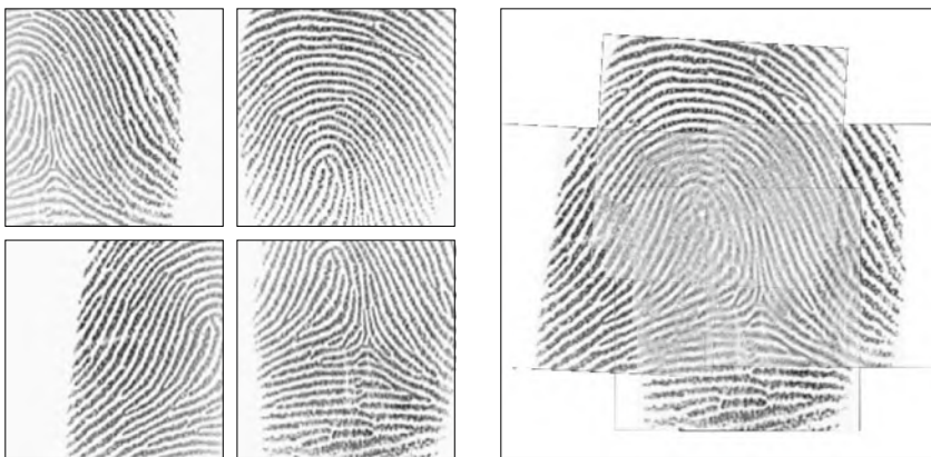
Fig. 2.29 A fingerprint mosaic image obtained by combining four fingerprint images acquired with a 0.51 \times 0.51 square inch 500 dpi optical sensor
