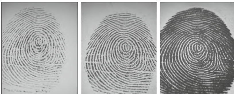
Fig. 7.18 Three impressions of the same real finger as captured when the finger is dry, normal, and wet, respectively. © IEEE. Reprinted, with permission, from Cappelli et al. (2002)
