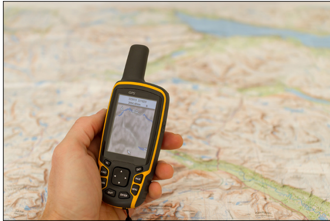
FIGURE 7-2: A typical handheld GPS device.
