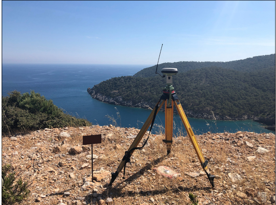
FIGURE 7-1: A typical GNSS base station.
