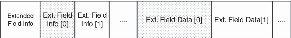
Figure 13.4 Extended field structure.
