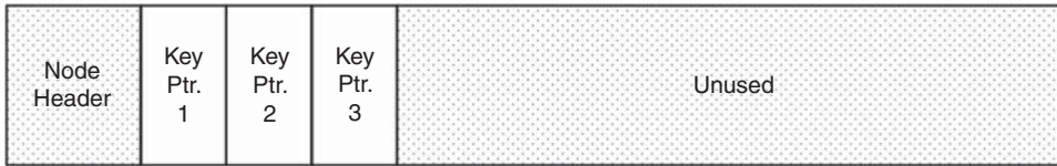
Figure 11.2 Btrfs B-Tree internal node structure.
