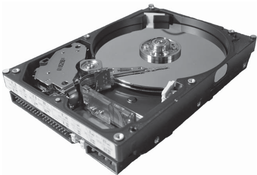
Figure 4.1 A traditional HDD with the cover removed showing the internal structure.
