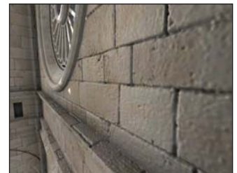
Figure 14.22: Voxel data created by high-resolution surface displacement, with local shadowing precomputed and stored in the voxel grid. The resolution is approximately 5 mm throughout the entire building, including outer walls that are not visible from the inside. The total size of the data in GPU memory is 2.7 GB. Laine and Karras's ray caster was able to cast about 61 million rays per second when rendering this scene; in other words, to render 1M pixels at 60 fps by ray tracing in 2010 [LK10]. (Credit: Courtesy of Samuli Laine and Tero Karras, © 2010 ACM, Inc. Reprinted by permission.)
