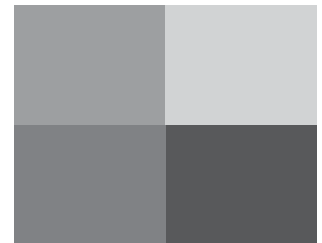
Figure 18.19: The values in a 2 \times 2 grayscale image are convolved with a box function to get a piecewise constant function on a 2 \times 2 square.
