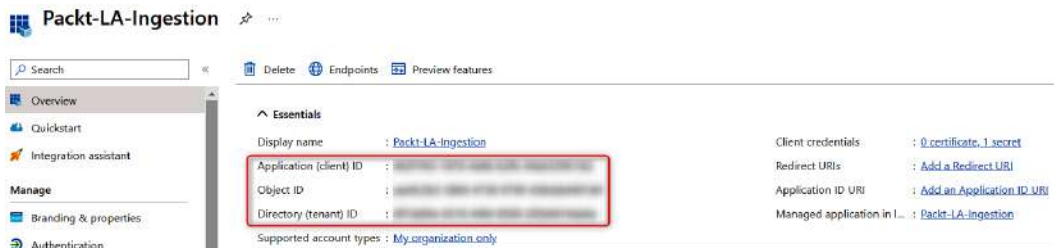
Figure 3.15 – Application registration for Logs Ingestion API call
