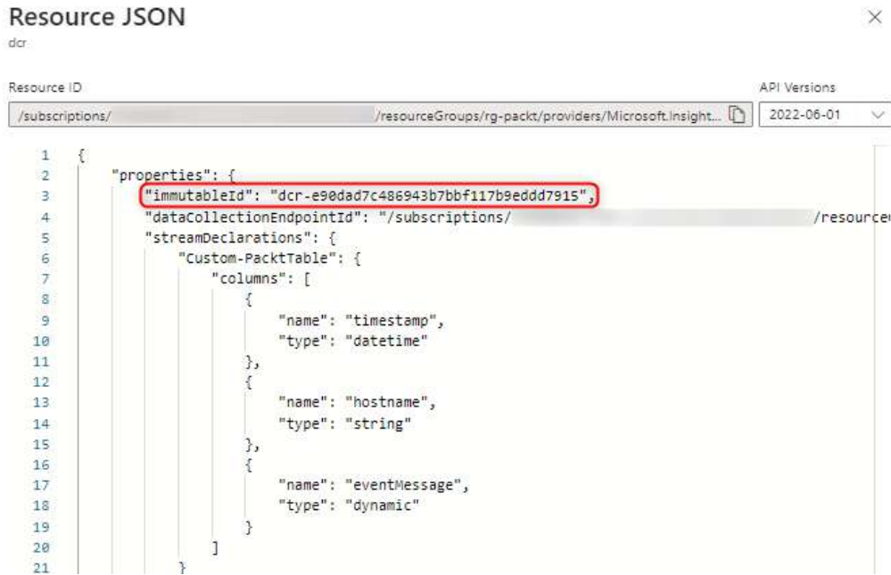
Figure 3.19 – The JSON definition of the DCR and the immutable ID property
