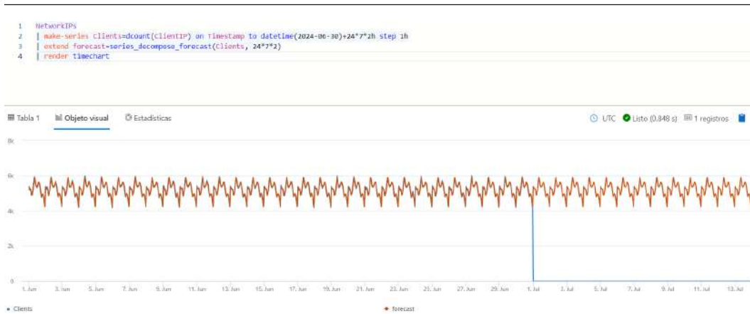
Figure 12.1 – Network IPs forecasting scenario using the series_decompose_forecast operator
