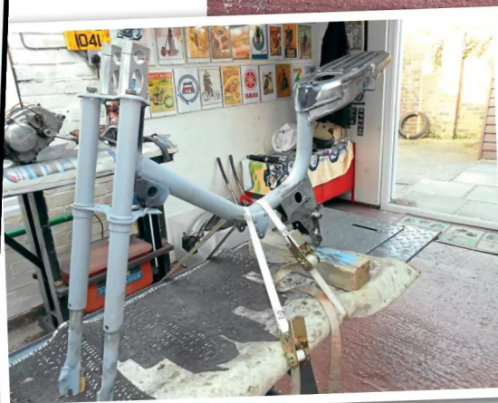
Amigo frame and the first task was to remove unwanted metal plus modify the rear panel and seat post
