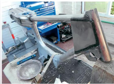
Tank securing tube and bracing plates
