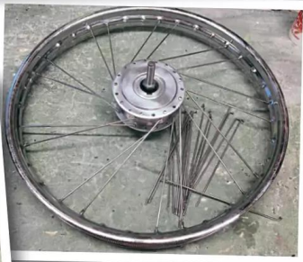
Rims and spokes supplied by Mopedland and built by Neil at Walton Works
