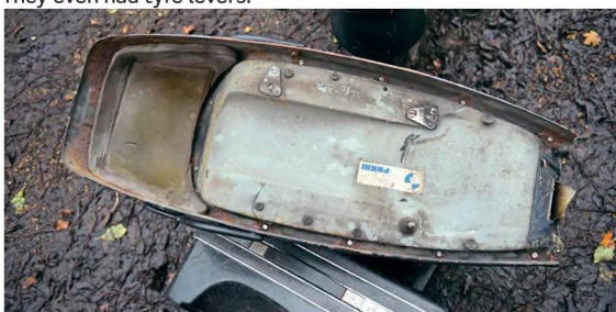
Seat has been recovered and base is glass-fibre – shell is steel and recoverable
