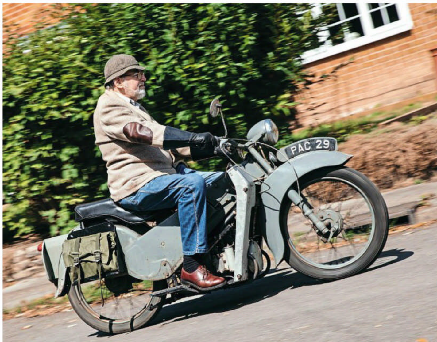
LE 192cc sv l/c flat twin || 250lb || 100+mpg || 55mph || 1949-71
