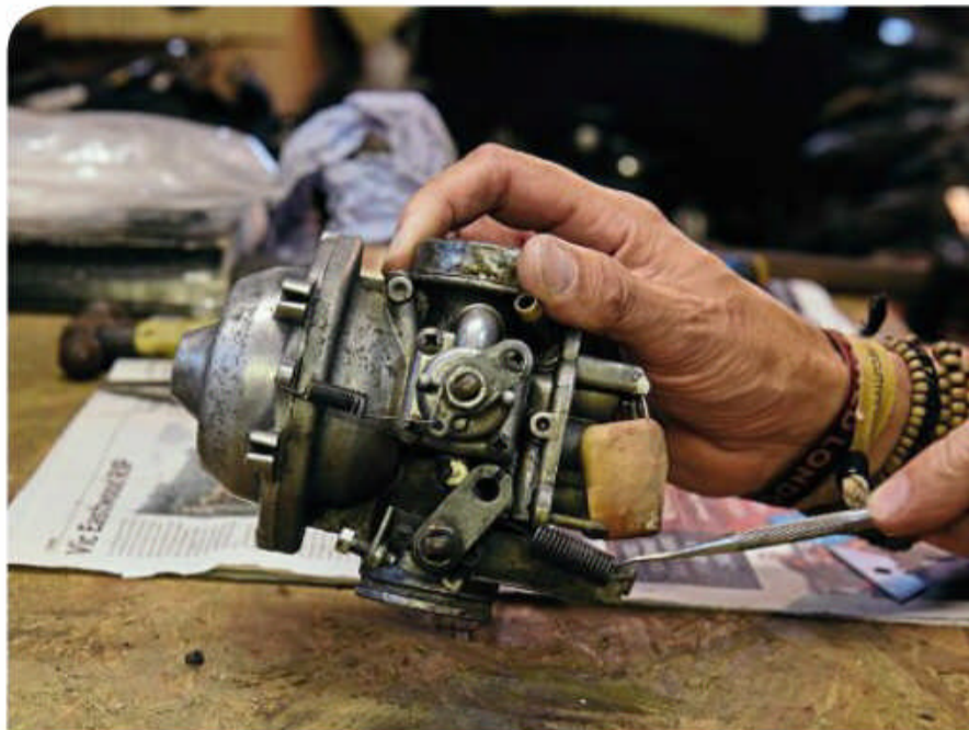
The mixture screw needs to be adjusted before running. The Clymer manual recommends just ¼ of a turn from full in, whereas the UK Haynes manual opts for ¾ to 1 full turn out (for the 32mm model). These are only a guidance, but it's close enough for it to start up. Make sure return springs are fitted too.
