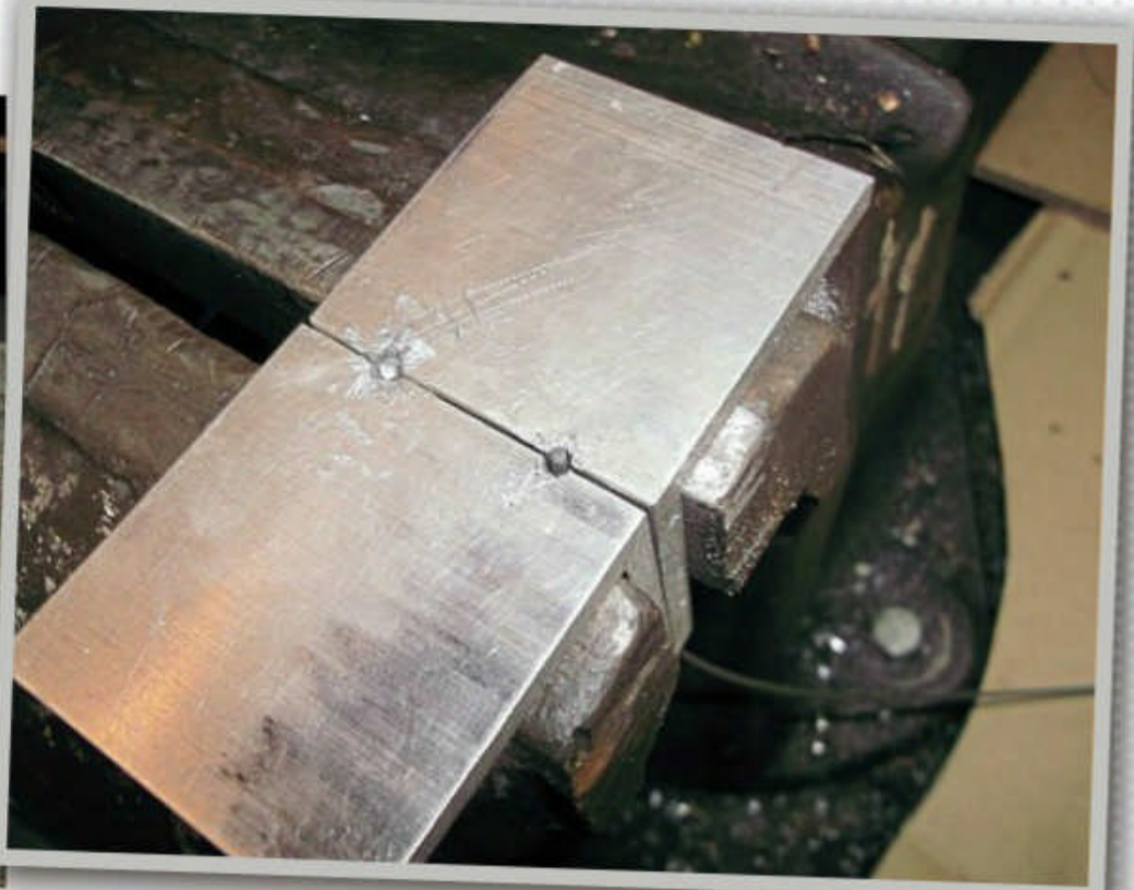
A simple jig to hold the cable in the right place so you can make a 'nest' at the end.
