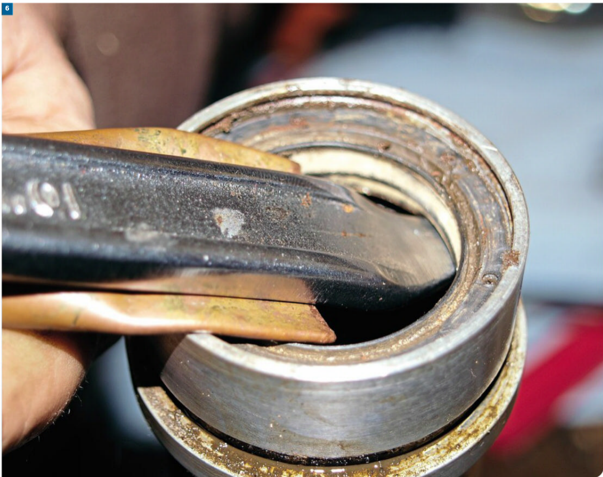
5. Everyone has their own preferred method of removing fork seals, but I've found a decent length tyre lever works well. Note the piece of squashed 22mm copper pipe under the lever protecting the thin wall of the seal's seat.
