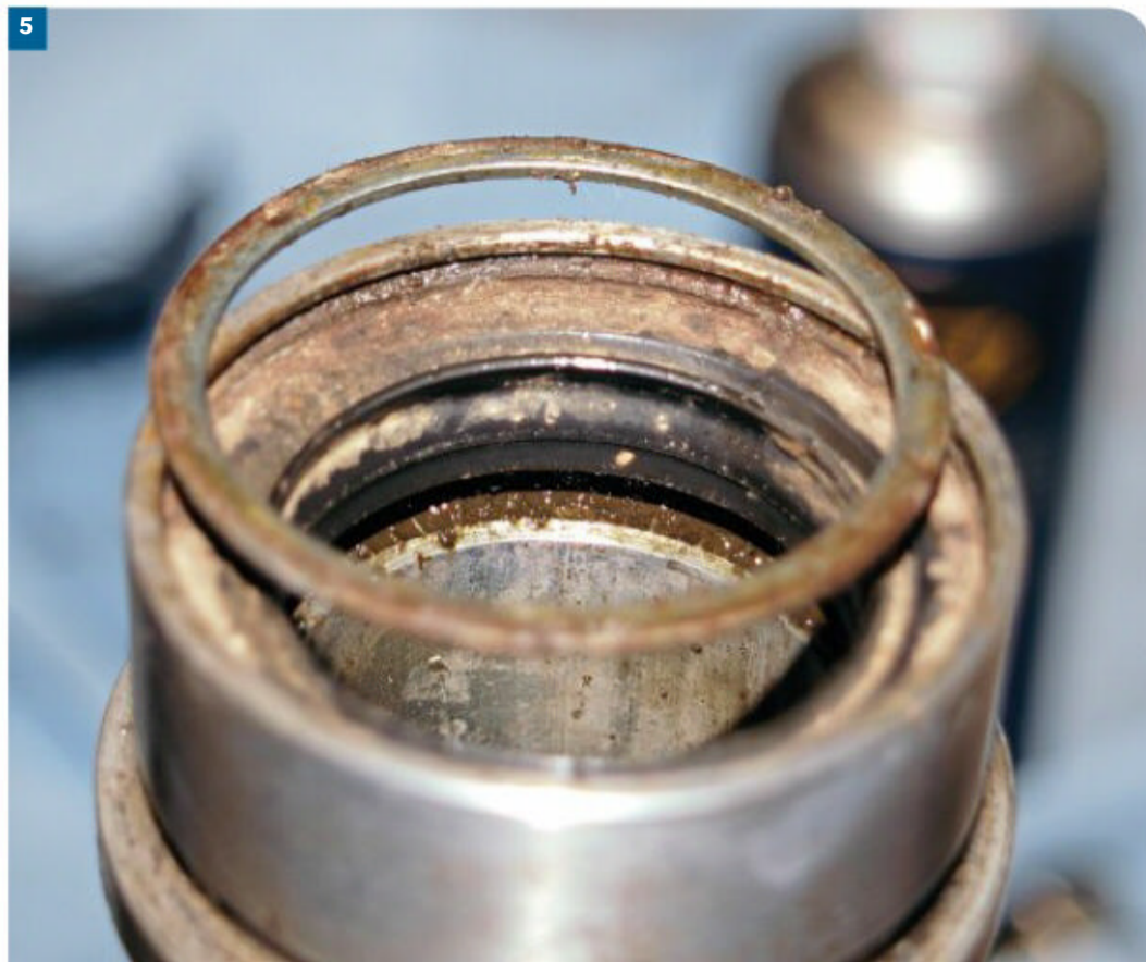
5. Everyone has their own preferred method of removing fork seals, but I've found a decent length tyre lever works well. Note the piece of squashed 22mm copper pipe under the lever protecting the thin wall of the seal's seat.
