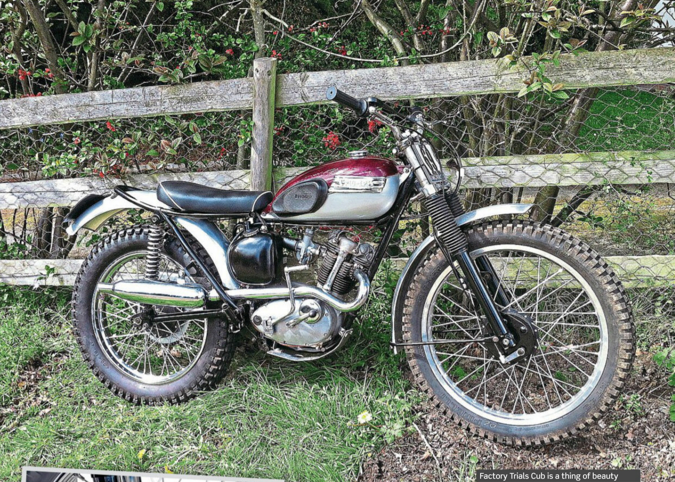
Narrower tank helps slow speed balance
