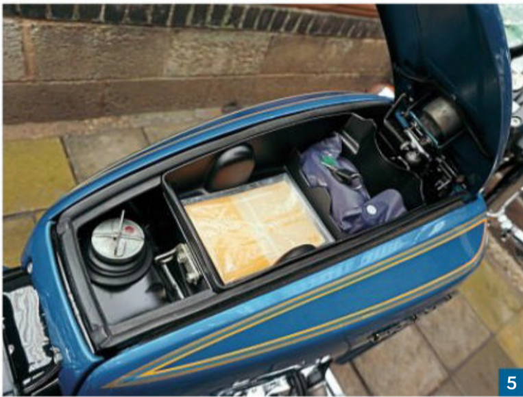
6. The right-side of the faux fuel tank. No, that metal bar isn't for self defence, that's the kick-start lever - re-zinc'd - which fits into a socket on the left-side near the gearbox. We also see the header tank and top-up cap for the water. The black screw locating knobs were later altered.
