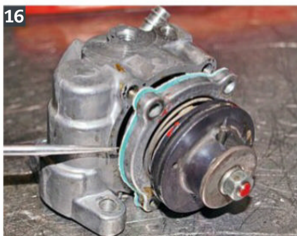
16: Replace the pump pulley housing onto the main body using a new gasket but do not add any silicone jointing compound or similar which would be highly likely to block the pump.
