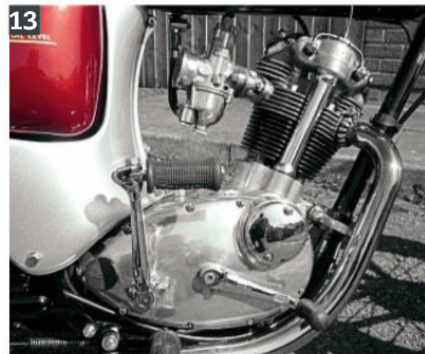
13: The later Amal 622, and now the points are behind that neat round chrome cover.
