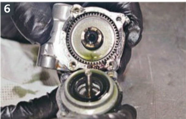
6: Inside we can see the driven gear wheel and some of the grey detritus that's built up on the central boss. Don't be tempted to remove components willy-nilly, for reasons that will become apparent shortly. Clean the insides and remove all of the old gasket.
