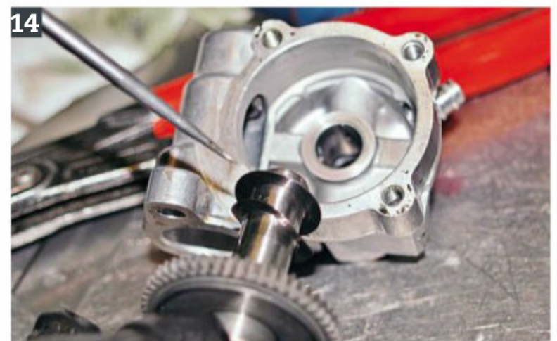
14: Now to rebuild everything starting with the end plate and driven wheel; it's vital that the shim and wave washer go back and in the correct order. Lubricating the components dramatically helps but it can still be a struggle....
