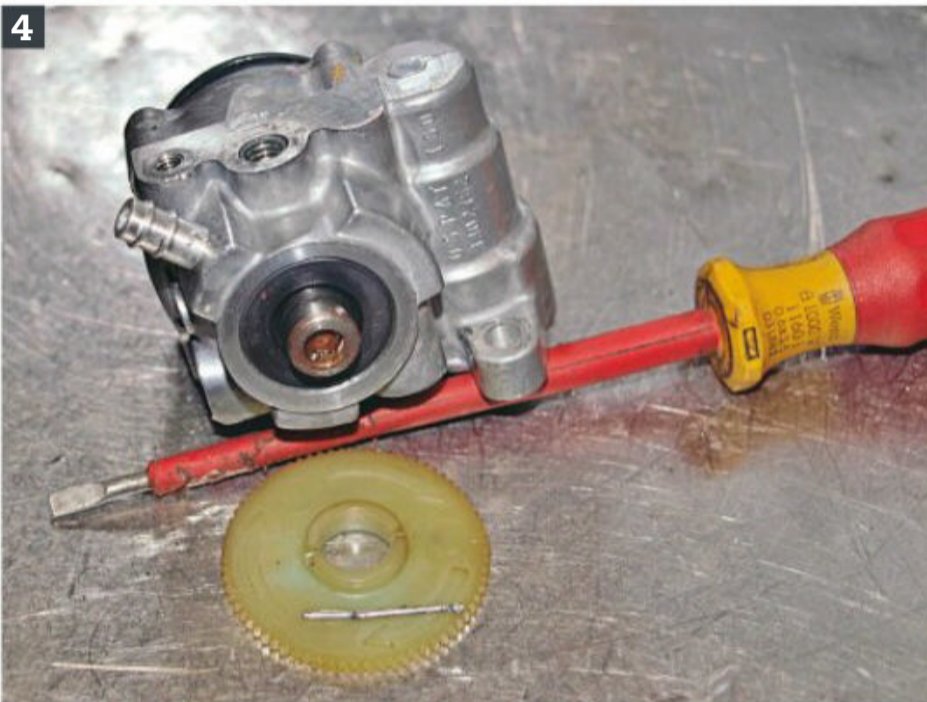
4: Remove the priming thumb wheel but ensure the pin is kept safe, it's an odd size and, annoyingly, not readily available.
