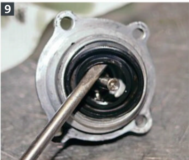
9: Note the seal's orientation and depth to which it was fitted BEFORE removing it from the pump top! Carefully prise out the old seal then clean.
