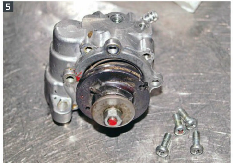
5: Using a decent quality screwdriver remove the four screws holding the pump together then pull the front end of the pump away from the main body. A gentle tap with small hammer will help to break the gasket's bond.
