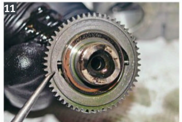
11: Sitting inside the drive gear are two tiny spring-loaded pins that act as part of a freewheeling mechanism. DO NOT DISASSEMBLE with very good reason. The pins and springs have a well-deserved reputation for flying out and getting lost. Simply spray with brake cleaner and allow to dry.
