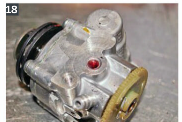
18: Replace the ball bearings and springs then add some two-stroke oil, temporarily holding everything in place with the banjo bolts. Bolt the pump back in place using a new gasket. Reconnect both the supply pipe and delivery tubes (using fresh fibre washers) then bleed the pump.
