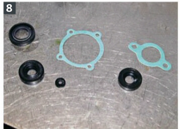
8: A typical Yamaha oil pump overhaul kit. Ours come from Alisdair Cowan of YDS Parts. Whatever you use ensure it's high end quality, not cheapo... your engine is depending on the pump!
