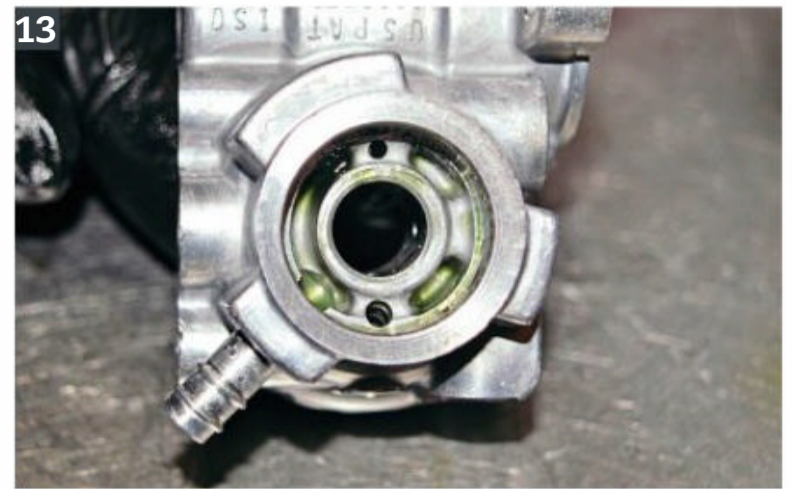
13: With the seal popped out we can wash away the goop that's accumulated at the lowest end of the pump. Most is of what's here is liquid but some is old, jellified, oil. Once clean the new seal is pressed in place.
