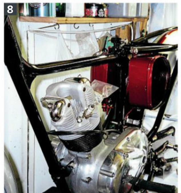
8: The neat little engine with its polished rocker covers is back in its frame. Toolbox and oil tank look resplendent in Chilli red
