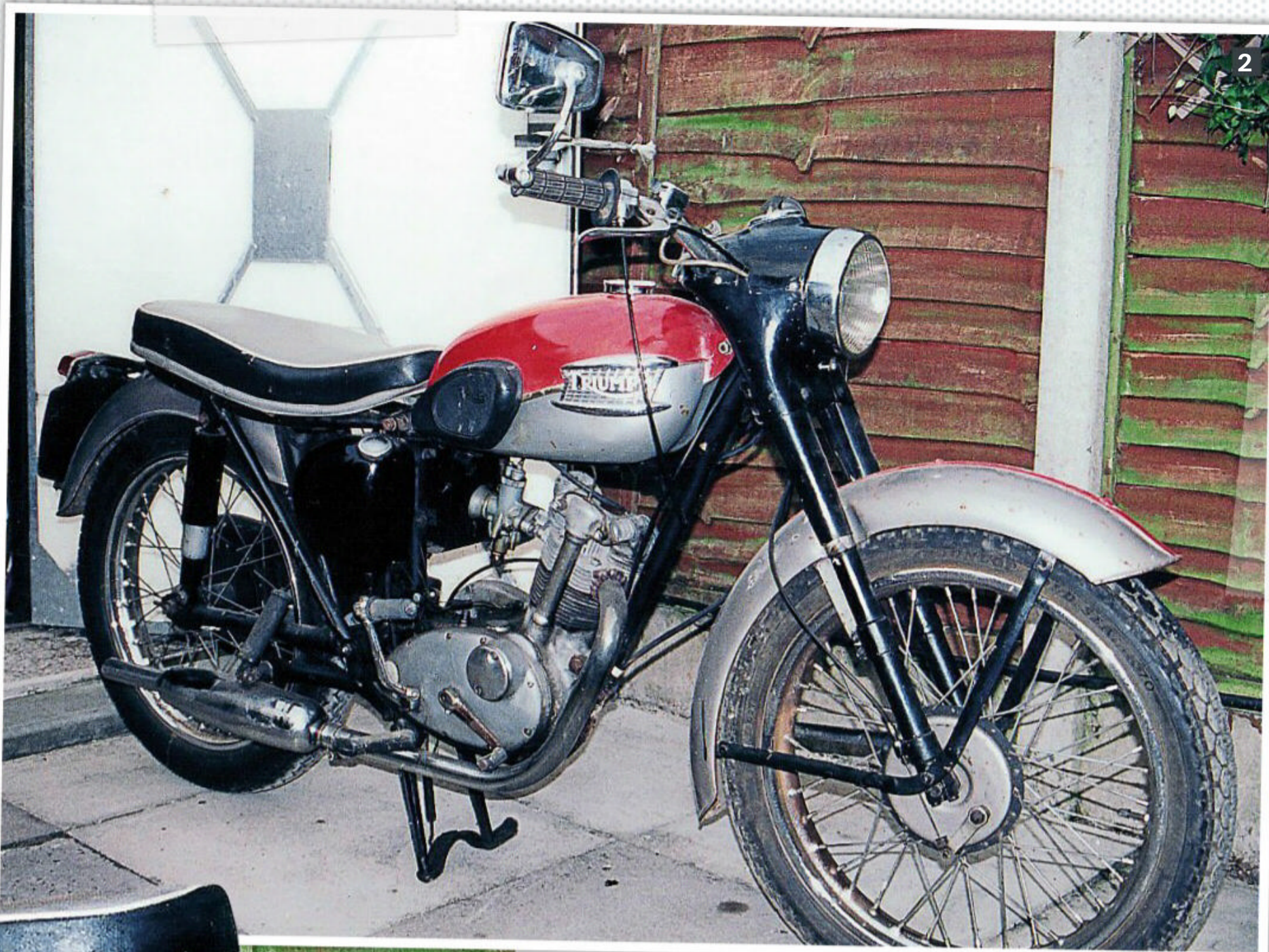
1 & 2: The Cub as purchased in 2004. Most parts are original and in situ, but not the bikini panels, which are so hard to obtain. Traditional Triumph knee pads and mouthorgan badge.
