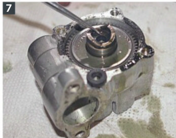
7: Indicated by the screwdriver is a seal that's easily overlooked, a new spare is towards the front. This seal should always be changed.
