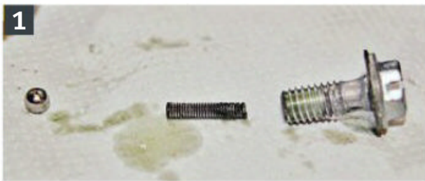
1: Beneath each banjo bolt is a spring and ball bearing; these stop the tank emptying its contents into the crankcases. Clean and safely store ready to use.
