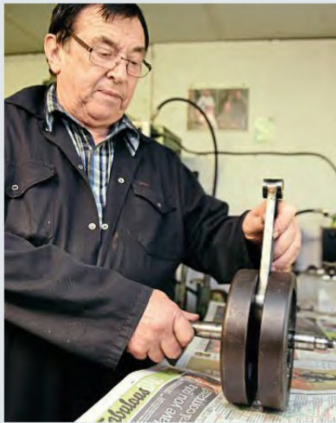
Trevor uses a breaker bar to undo the crank pin nuts, but finds they are loose!
