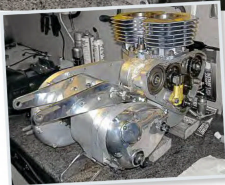
Above: Norton clutch and belt drive and also up rated alternator
