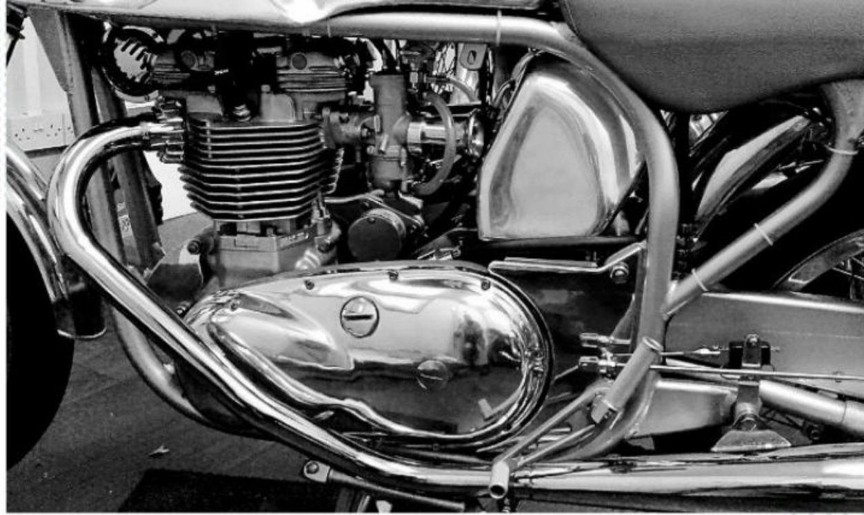
Above: If you look carefully, the primary case has had an extra viewpoint for clutch adjustments
