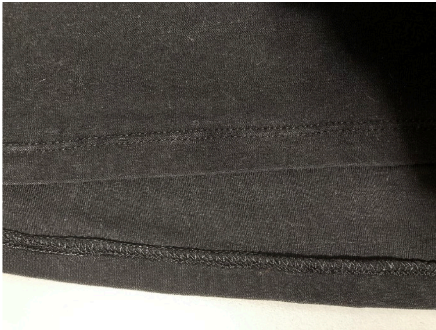
Hem by overlocking the edge and topstitching using a double needle
