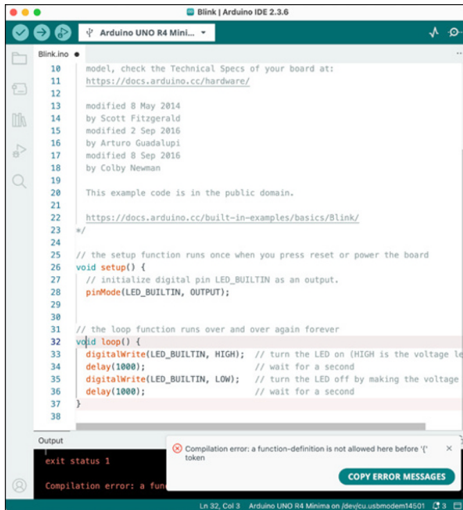
FIGURE 3-8: The Arduino software is telling you that a bracket is missing.
