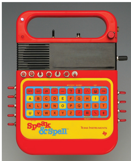
FIGURE 1-5: A Modified Toy Orchestra Speak & Spell after circuit bending.
