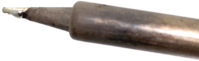
FIGURE 9-17: Tinning the tip helps to preserve your iron and makes soldering easier.
