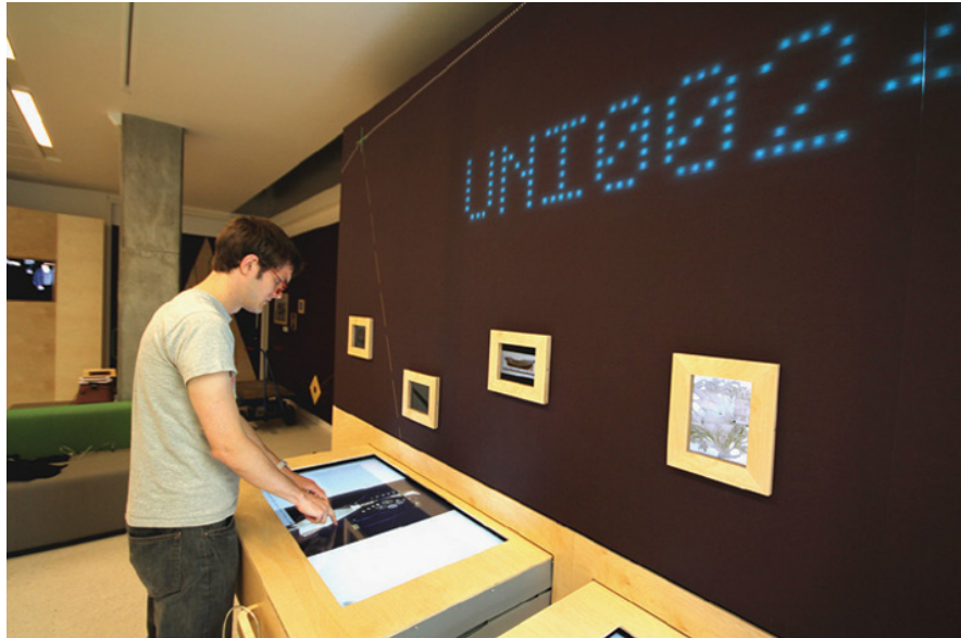
FIGURE 8-4: The hidden LED display lights up underneath the wallpaper.
