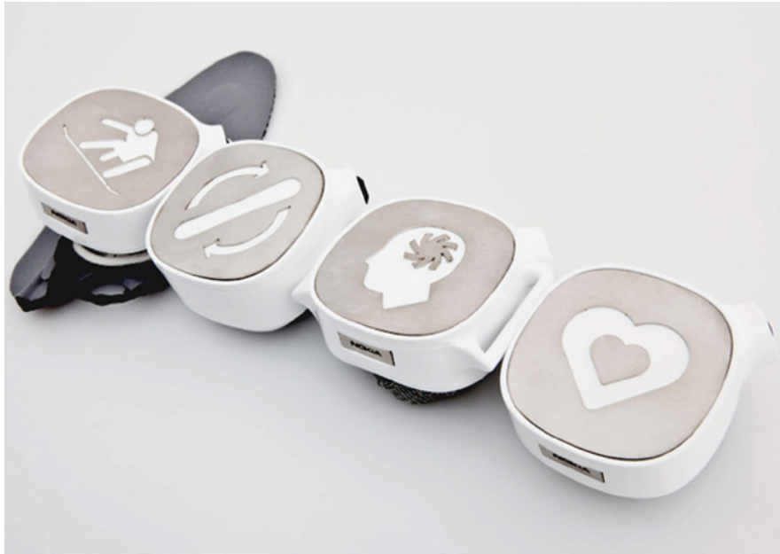
FIGURE 8-2: Snowboarding sensors in customized sensor boxes.
