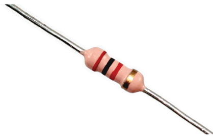
FIGURE 5-10: The color bands on a resistor.
