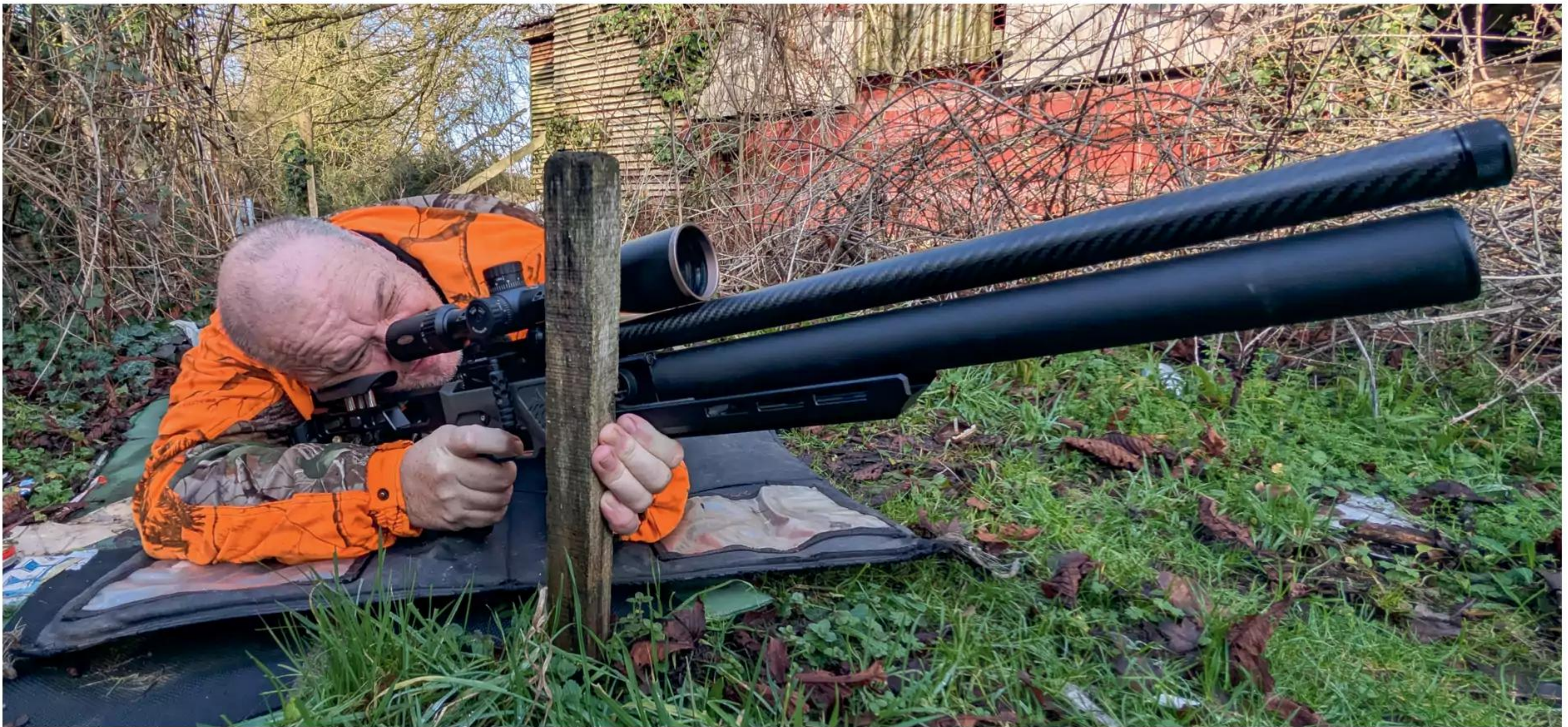
The adjustable comb on the Zero Tactical makes eye alignment easy on this large rifle
