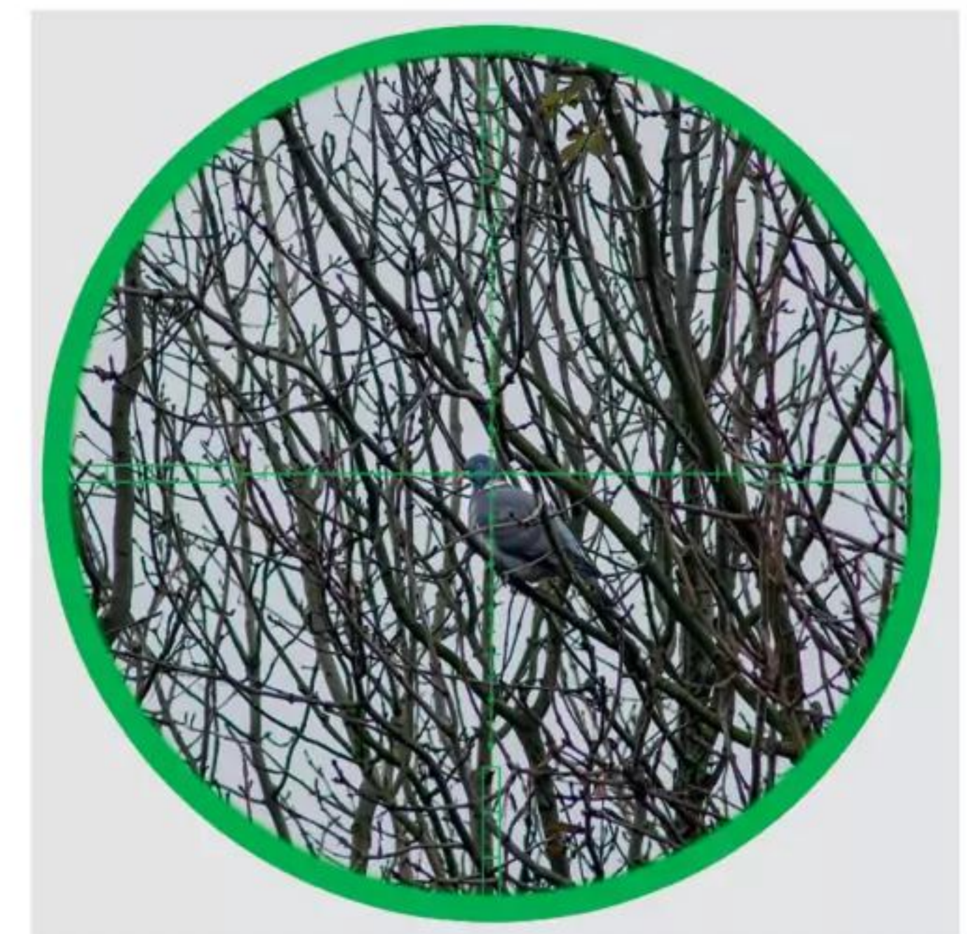
Below and opposite: The Wild's SFP crosshair offers plenty of aiming points and is illuminable to one of five intensities in either red or green. This makes it ideal to pick out against all types of target scenarios
